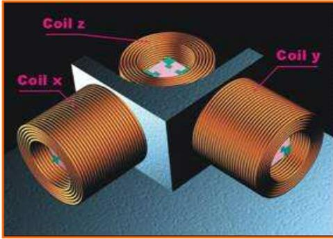
**Figure 4.** Overview of the three dimensional hard Hall probe assembly, showing the coils wound around the three hall sensor .
