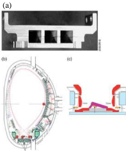
**Figure 5** a) The cassette assembly containing the mirror materials, b) c) the locations of the mirror test units inside JET vacuum vessel.
