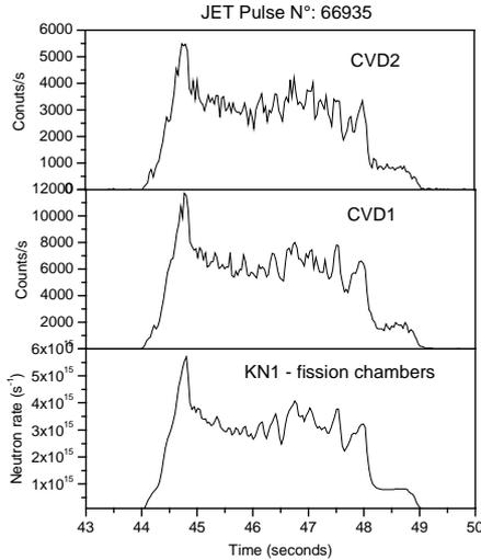
**Figure 3.** Comparison of time dependent neutron emission measured by fission chambers, and two types of CVD diamond detectors: polycrystalline (CVD1) and monocrystalline (CVD2) during JET Pulse # 66935.
