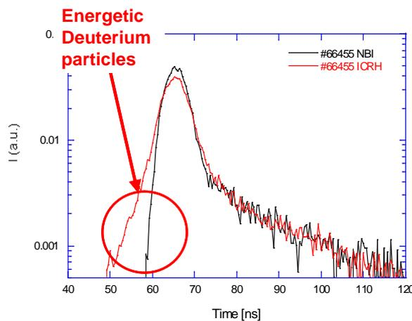
**Figure 2.** Neutron emission spectra measured with TOFOR from JET discharge #66455 during a phase with NBI (black) and during a phase with ICRH heating (red).
