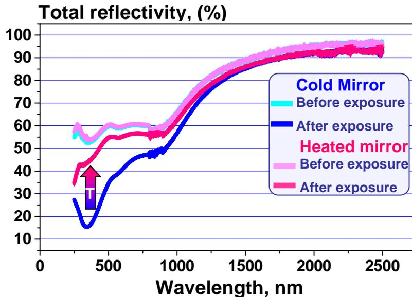
Figure 2: The evolution of the total reflectivity of molybdenum mirrors before and after exposures in DIII-D divertor. The data from [8] is used.
