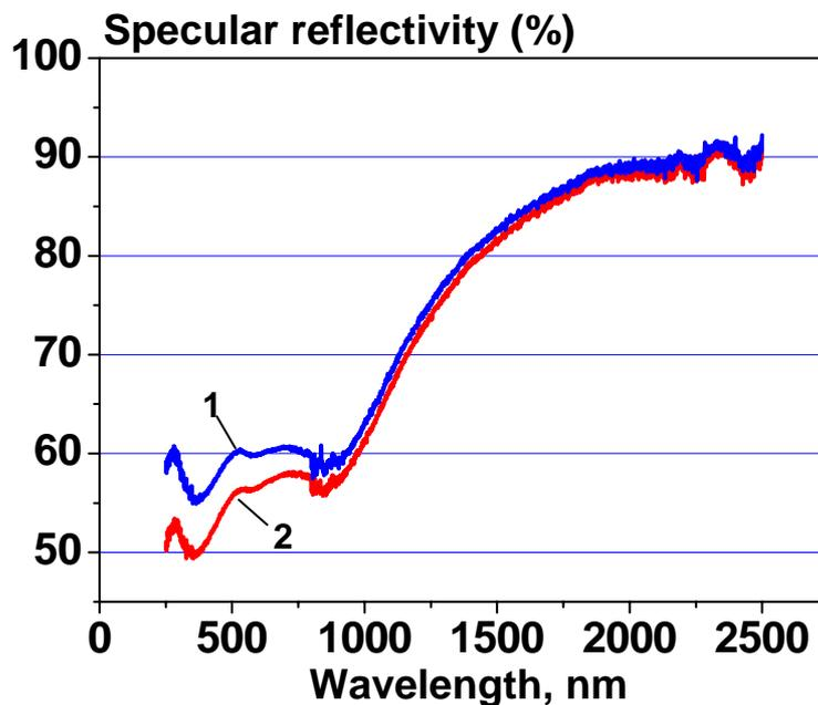
Figure 1: The specular reflectivity of molybdenum mirror after exposure in TEXTOR:
