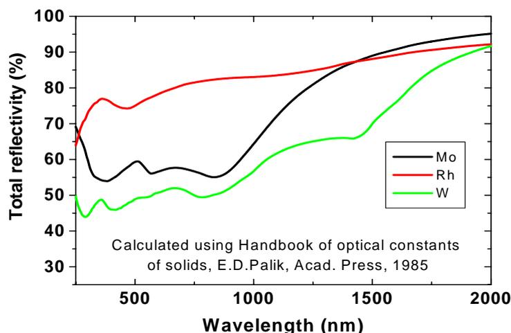
Figure 4 . The reflectivity as a function of a wavelength for molybdenum, tungsten and rhodium mirror materials.
