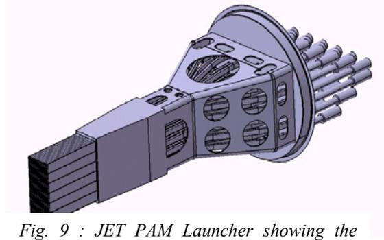
Fig. 9 : JET PAM Launcher showing the mechanical structure which holds the wave guide array from the back flange
