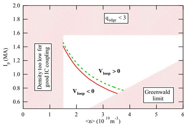
Fig. 4: plasma current vs. mean plasma density for the 30 s pulsed (green dashed curve) and steady state (red solid curve) scenarios.
