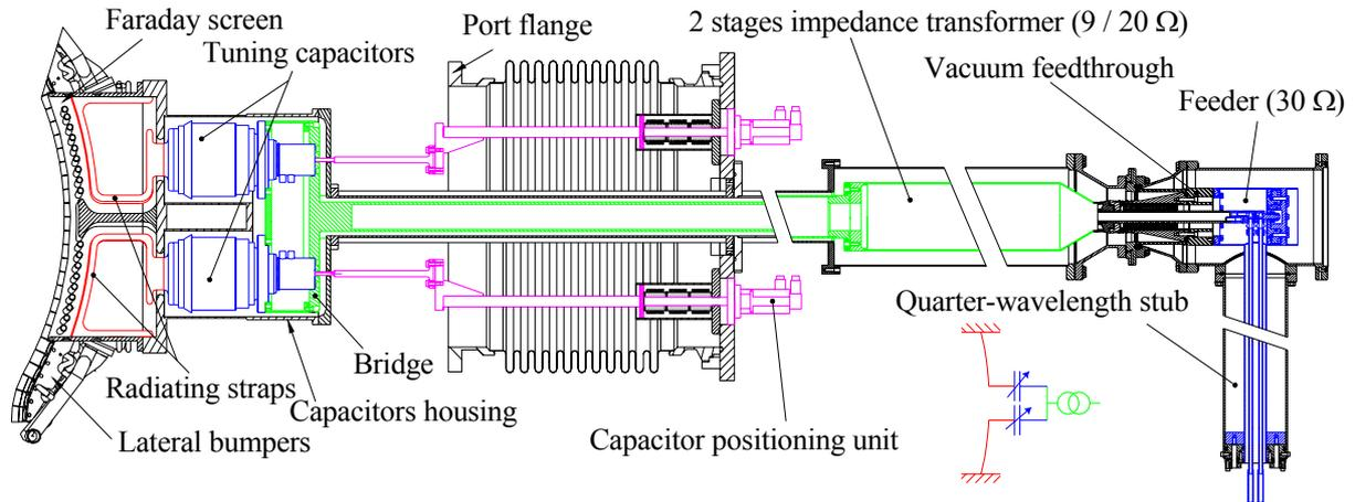
**FIG. 7 :** Layout of the ITER-like antenna prototype tested in 2004, featuring in color the different subsystems. red : radiating straps; green : vacuum feed ( $9\Omega$ ) and 2-stage impedance transformer ( $9/20\Omega$ ); blue : tuning capacitors ; dark blue : quarter wavelength stub ; magenta : capacitor positioning units.
