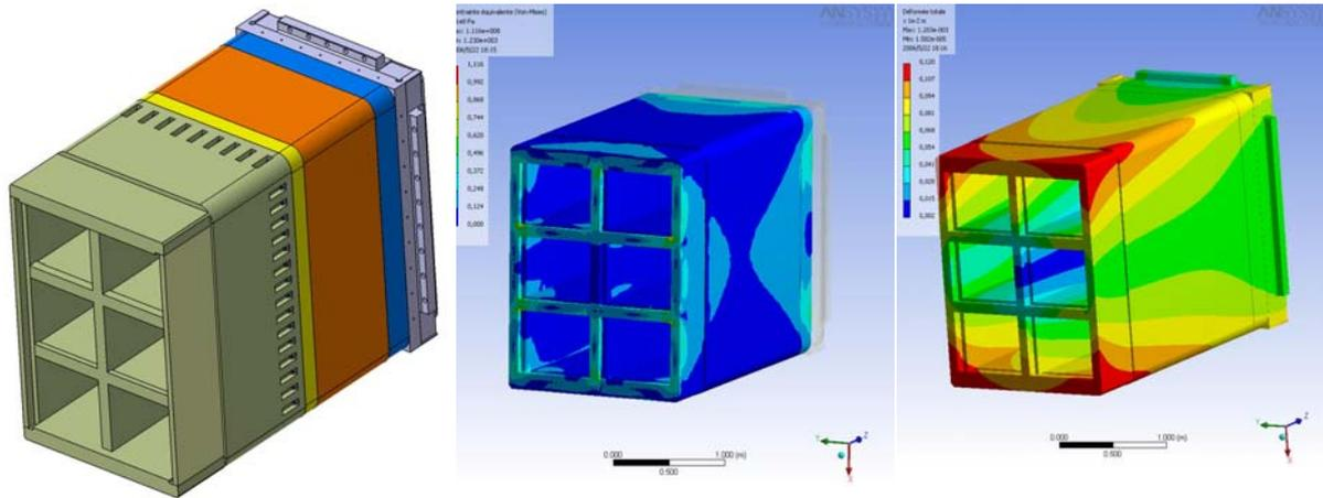
Fig.10 : a) Plug overview, b) Stress distribution Von Mises Max=116 MPa c) deformation (Max= 1.2mm)
