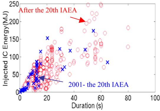
Fig. 1: Injected ICRH versus pulse duration; operations circles = during the last two years; crosses = before the 20<sup>th</sup> IAEA
