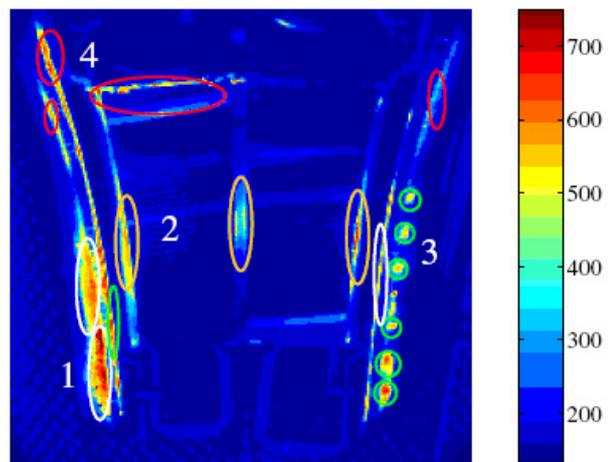
Fig. 3 : IR image of IC antenna, at  $t = 63.7\text{s}$ , in a combined ICRH (4MW)/LHCD (3MW) discharge (Unit is  $^{\circ}\text{C}$ ,
