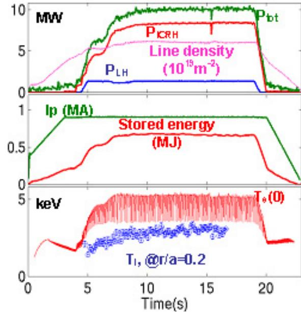
Fig. 2: shot 33612, Combination of ICRH (8.5 MW) and LHCD (1.4MW)
