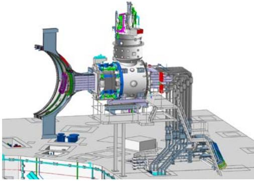
Fig.8: PAM launcher as inserted in JET port, fed by its 36 waveguides transmission line
