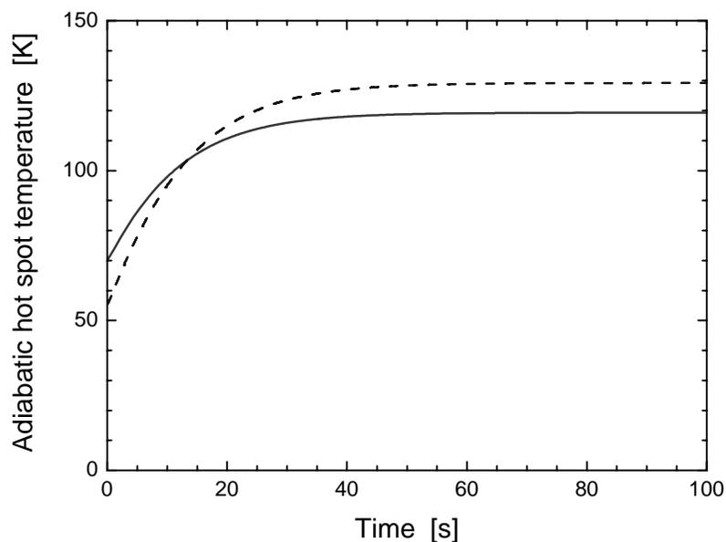
FIG. 1. Temperature rise during a safety discharge for the two sample conductors. Here an YBCO layer thickness of  $1 \mu\text{m}$ , and a Cu stabilizer thickness of  $50 \mu\text{m}$  (solid line) and  $300 \mu\text{m}$  (dashed line) have been used.
