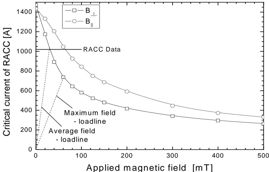
FIG. 3. Critical current characteristic of MOCVD-CC (Superpower) with field orientation parallel and perpendicular, scaled up to the RACC-cable design current of 1467 A. The load lines from self field effect calculations (see text) intersect the worst  $I_c(B)$  curve at 1040 A and 736 A for the different approaches. The very good agreement using the average field approach indicates a very well working current redistribution.
