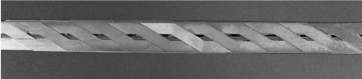
*FIG. 2. View of the 16 strand ROEBEL assembled coated conductor (RACC) made from DyBCO-CC (THEVA), Cable dimensions 10 mm width, 1 mm thickness and 180 mm strand transposition length*
