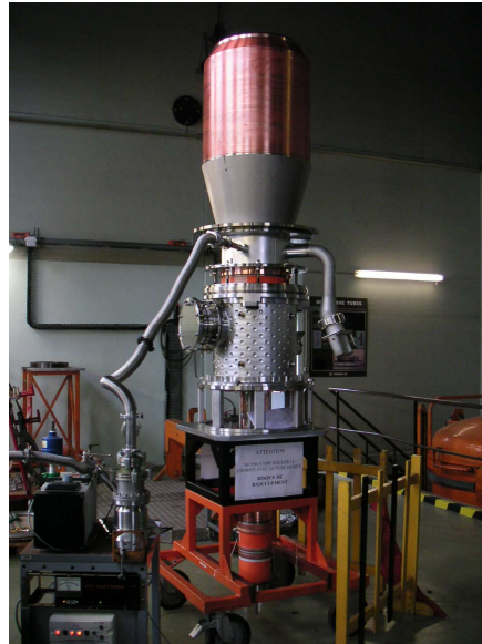
FIG. 6. 2MW-170 GHz prototype produced by THALES Electron Devices
