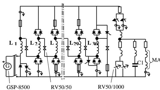
Fig.4. A circuit of the first two stages of the MOL module
