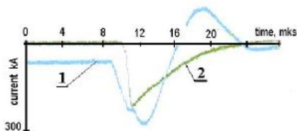
Fig. 10. PCS operation with a prepulse. 1 - current at the PCS inlet, 2 – current on load.
