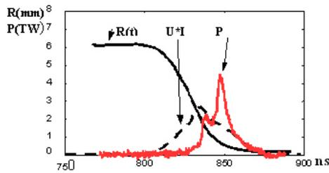
Fig. 3. Profiles calculated in terms of current and voltage measured. Y-axis:  $U \cdot I$  [TW] is the electric power input  $r_0$ ,  $P$  [TW] is the X-ray power and  $R$  ( $r$ ) (mm) is the average current radius,
