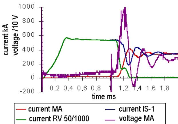
Fig.6. Current and voltage oscillograms at the energy transfer from IS-1 to MA
