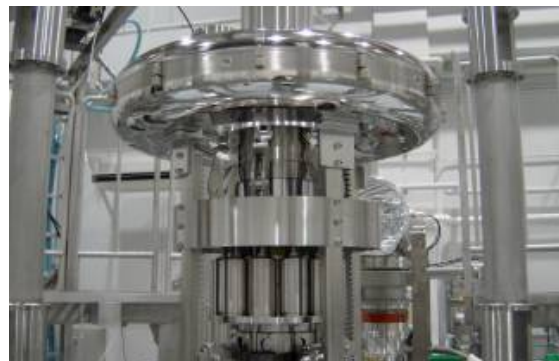
FIG. 6. The super-conducting ring magnet supported by the lifter. The catcher system is installed on the center column.
