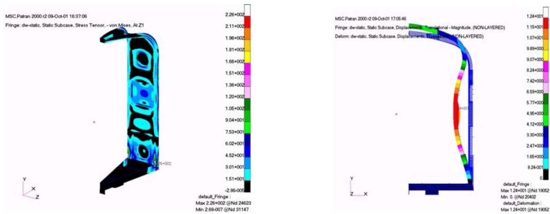
FIG.6. Stress Analysis for Cryostat
