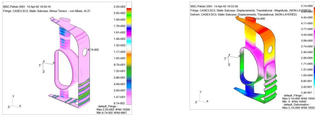
FIG.5. Thermal Stress Analysis for Thermal Shields
