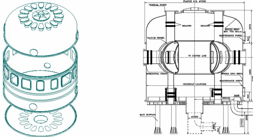
FIG.3.The Structure of Cryostat
