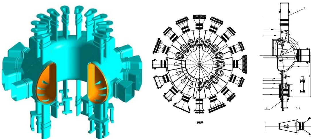
FIG.1. The Structure of Vacuum Vessel
