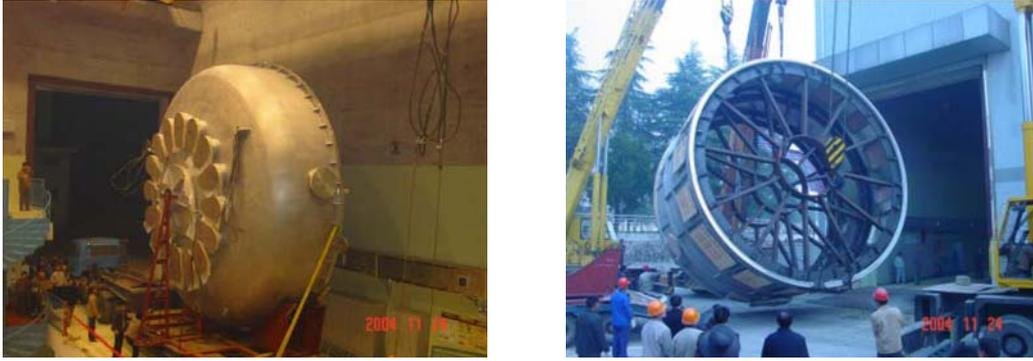
FIG.9. Fabrication of Cryostat
