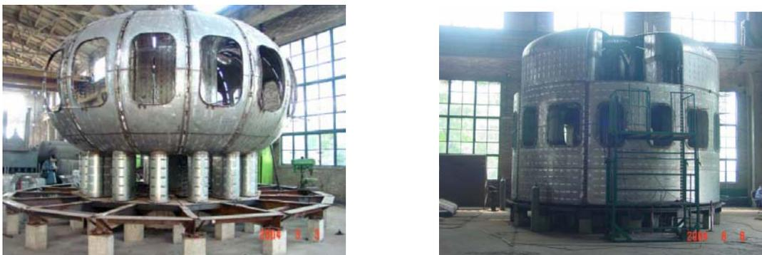
*FIG.8. Fabrication of Thermal shields*
