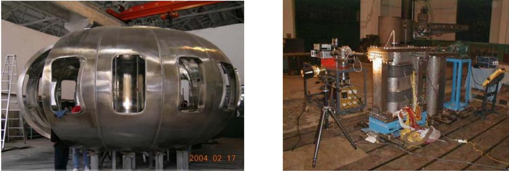
*FIG.7. Fabrication of Vacuum Vessel*
