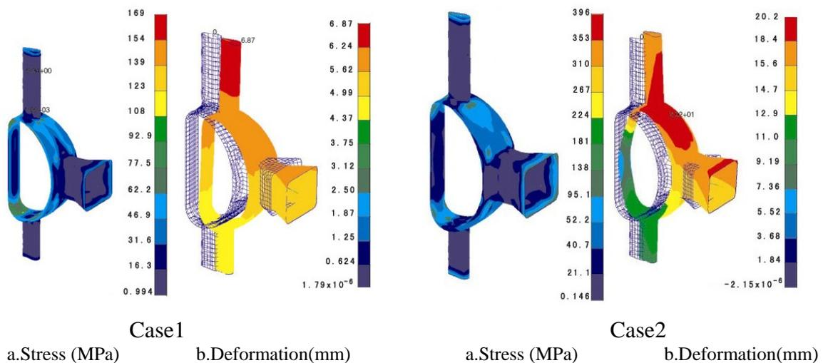
FIG.4. Maximum stress and deformation of the vacuum vessel
