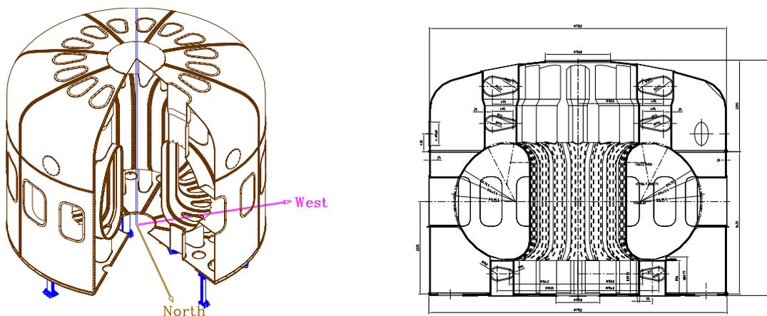
FIG.2. The Structure of Thermal Shields
