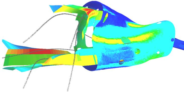
*FIG. 2: Heat loads on the W7-X plasma vessel and divertor structure by plasma radiation emitted from the X-Points (scattered gray line). The color indicates the heat-flux, red  $130 \text{ kWm}^{-2}$  down to blue  $0 \text{ kWm}^{-2}$ .*
