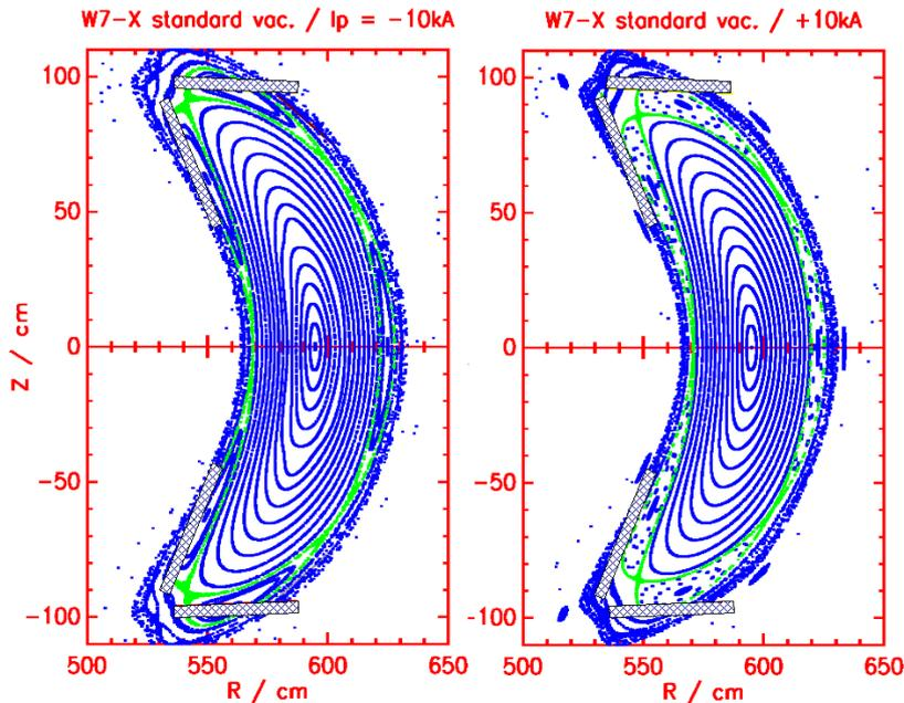
FIG. 1: W7-X standard magnetic configuration for different bootstrap current values ( $\pm 10$  kA). The green point indicate the separatrix. The X point distance to the target plates (shaded area) varies like  $2.5\text{mm} / \text{kA}$ .
