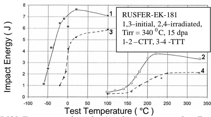
FIG. 6. RUSFER-EK-181. Temperature dependencies of impact energy of small specimens (v-Chardy-KLST) with different thermal treatments (1-2 – cyclic thermal treatment – CTT, 3-4 – traditional thermal treatment – TTT) before (1, 3) and after (2, 4) irradiation in BOR-60 reactor (radiation damage 15 dpa, irradiation temperature 340 °C).
