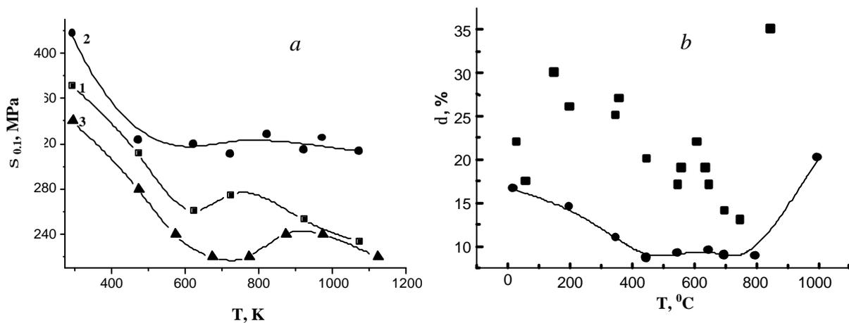
FIG. 10. V-4Ti-4Cr alloys (3 - USA, 1-2 - RF): (a) temperature dependence of the yield stress after traditional thermal treatments (1, 3) and after new thermo-mechanical treatment (2); (b) ultimate elongation of the V-4Ti-4Cr (RF) alloy after traditional (squares) and new (circles) regimes of thermal treatments.
