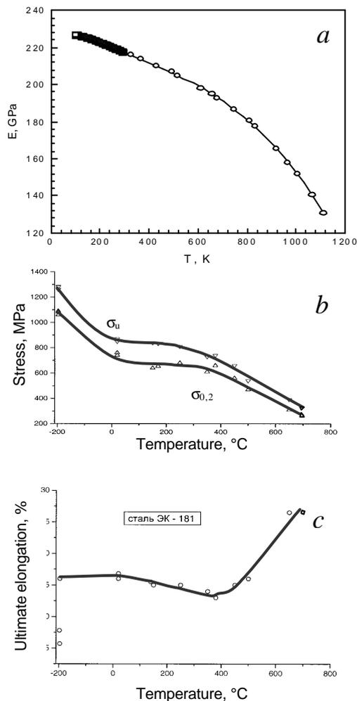
FIG. 3. RUSFER-EK-181. Mechanical properties of the specimens (TTT) vs. temperature curves: (a) elastic module (E, GPa), (b) yield point ( $\sigma_{0.2}$ , MPa) and ultimate stress ( $\sigma_u$ , MPa), (c) ultimate elongation (%).
