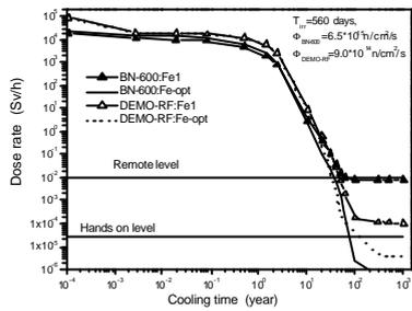
FIG. 2a. RUSFER-EK-181. Activity decay in "recommended" (Fe-opt) and manufactured (Fe1) compositions "irradiated" in BN-600 and DEMO-RF (irradiation time is 560 effective days in both cases).
