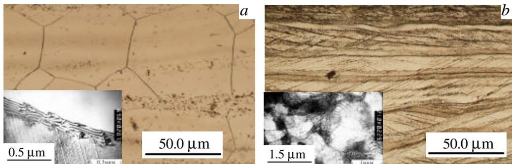
FIG. 9. Microstructures of V-4Ti-4Cr (RF) specimens: (a) traditional thermal treatment, (b) new treatment.
