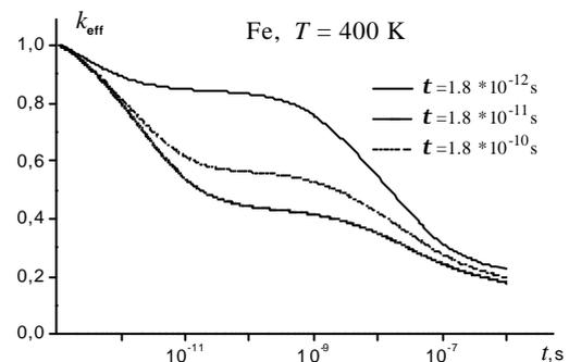
FIG. 1b. Factor  $k_{eff}$  of the defect formation by cascade (coefficient of the cascade efficiency) vs. time  $t$  (s) curves for different time ( $t$ , s) of the changing of thermal conductivity mechanism (phonon to electron) (Fe, the primary recoil energy  $E_{pr}=5$  keV, crystal temperature 400 K).
