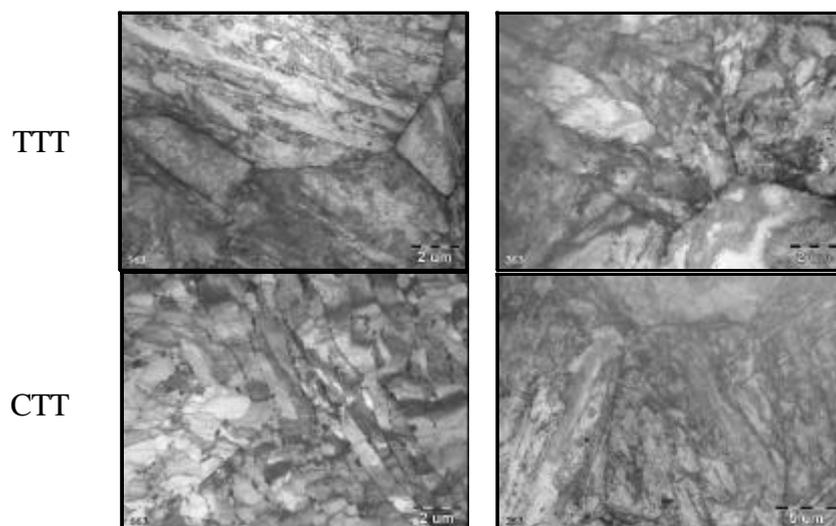
FIG. 7. RUSFER-EK-181. Microstructure of the specimens after traditional (TTT, upper row) and cyclic thermal treatment (CTT, lower row) before (left row) and after (right row) irradiation (BOR-60, 325 °C, 6 dpa).
