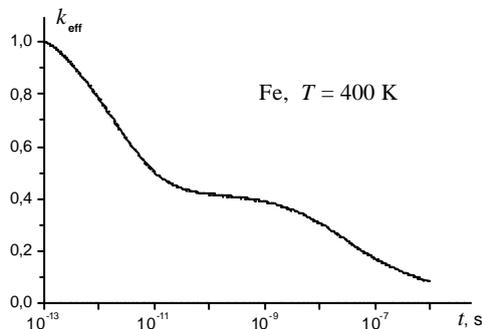
FIG. 1a. Factor  $k_{eff}$  of the defect formation by cascade (coefficient of the cascade efficiency) vs. time  $t$  (s) curve (Fe, the primary recoil energy  $E_{pr}=60$  keV, cascade formation time  $t=0$ , crystal temperature 400 K).
