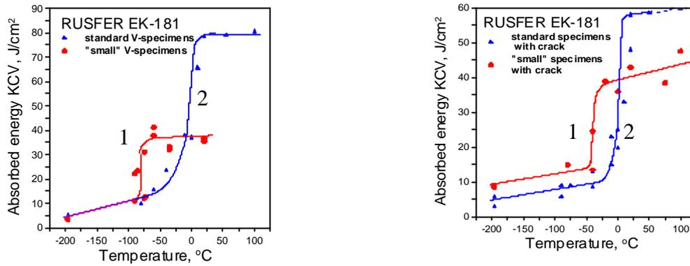
FIG.5. RUSFER-EK-181. Charpy impact energy vs. test temperature curves for small (1) and standard (2) specimens (TTT) without and with crack.
