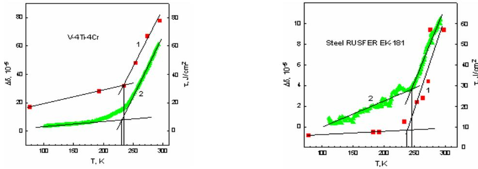
FIG. 8. Comparative behavior of impact toughness (1) and logarithmic decrement (2) with temperature for vanadium alloy V-4Ti-4Cr (left) and steel RUSFER-EK-181 (right) samples. One can see a good correlation of the both properties for both materials.
