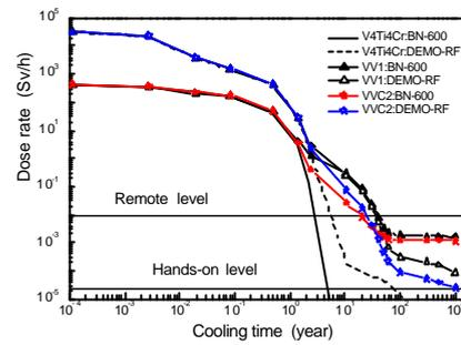
FIG. 2b. V-4Ti-4Cr. Activity decay for "pure" (V-4Ti-4Cr), recommended (VV1) and manufactured (VVC2) compositions "irradiated" in BN-600 and DEMO-RF (irradiation time is 560 effective days in both cases).
