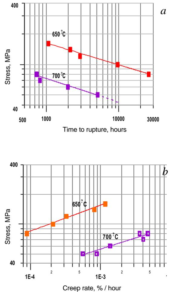
FIG. 4. RUSFER-EK-181. Time of the creep-rapture time (hours) (a) and creep rate (%/hour) (b) of the specimens (TTT) under temperature 650  $^{\circ}$ C and 700  $^{\circ}$ C in dependence from stress (MPa).
