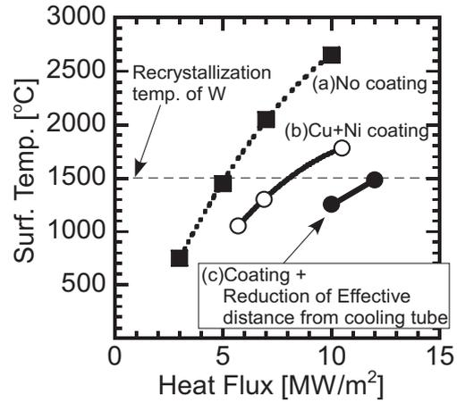
Figure 9. Comparison of thermal response of W-hot pressing mock-ups with different joining conditions in high heat flux experiment.
