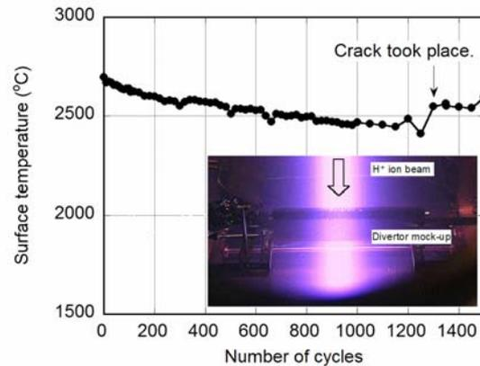
Figure 5 Maximum surface temperature evolution of the mock-up under the high heat flux condition of 20MWm<sup>2</sup>.
