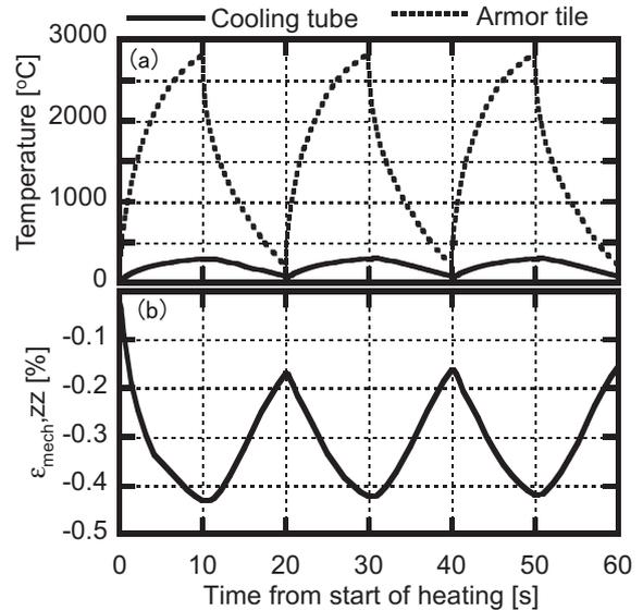
**Figure 7. Evolutions of temperatures of the cooling tube and the armor tile and mechanical strain of the cooling tube in the axial direction,  $\epsilon_{\text{mech},zz}$ , for three cycles at  $20\text{MW/m}^2$  for 10 s.**
