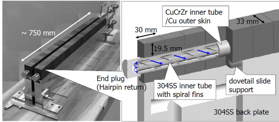
Figure 4 Schematic drawing and overall view of large-scale divertor mock-ups with a coaxial swirl tube.
