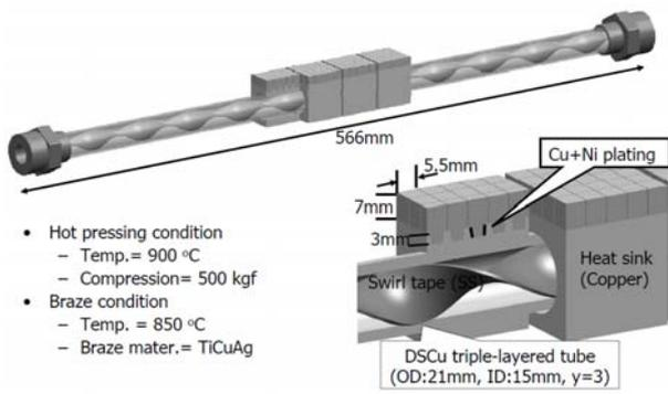
Figure 8. Schematic drawing of a divertor mock-up with pin-shaped tungsten armor.
