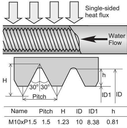
**Figure 1** Schematic view of screw tube made of F82H
