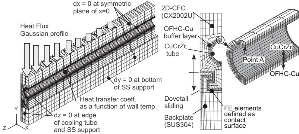
**Figure 6. Three-dimensional FEM model and boundary conditions for thermo-mechanical analyses of a large-scale divertor mock-up with a dovetail sliding support.**
