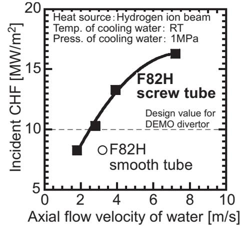
**Figure 2** Incident critical heat flux (CHF) of F82H screw tube.
