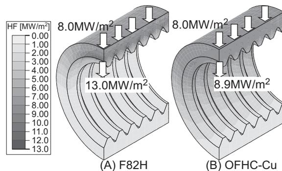
**Figure 3** Heat flux distribution inside the screw tube with M10 thread of 1.5-mm-pitch made of F82H and pure Cu at 8 MW/m<sup>2</sup>.
