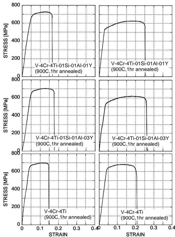
FIG. 4 Typical stress-strain curves for the V-4Cr-4Ti-type alloys after neutron irradiation at 450°C to the fluences of  $1.1 \times 10^{22}$  (left column) and  $2.5 \times 10^{21}$  (right column) ( $n/cm^2$ ,  $E_n > 0.1 MeV$ ).
