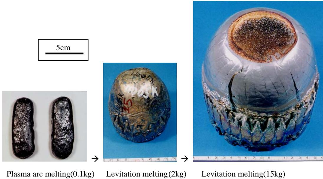
FIG.2. Scale-up of melting ingot of V-Cr-Ti-Si-Al-Y type alloys. Optimum procedure of melting procedures and chemical compositions were identified so far from various mechanical and compositional investigations.
