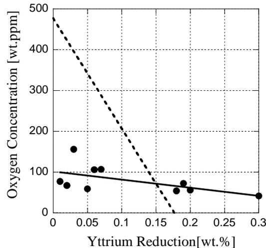
FIG.1. Correlation between oxygen concentration and amount of reduced yttrium in the V-4Cr-4Ti-Y alloys fabricated by levitation melting process. Dashed line represents calculated oxygen concentration when all of oxygen in the alloy removed as  $Y_2O_3$  slug formation. Initial oxygen concentration set same as in the V-4Cr-4Ti alloy without yttrium addition (480wt.ppm).
