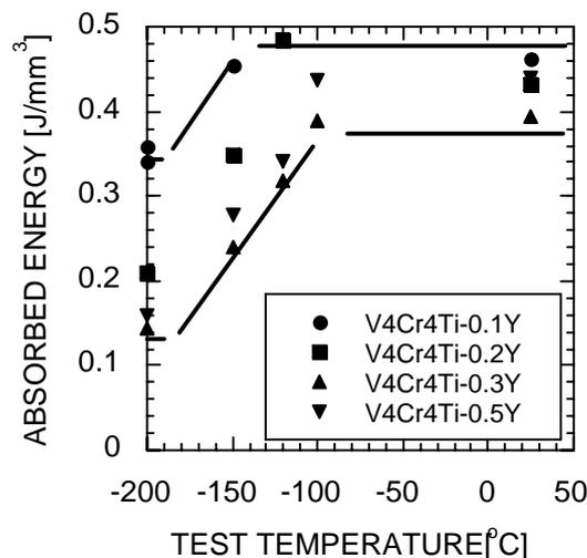
FIG.3. Charpy impact absorbed energy versus test temperature of V-4Cr-4Ti-Y alloys with various amounts of Y addition. Lower levels of yttrium addition shows higher absorbed energy at low temperatures.
