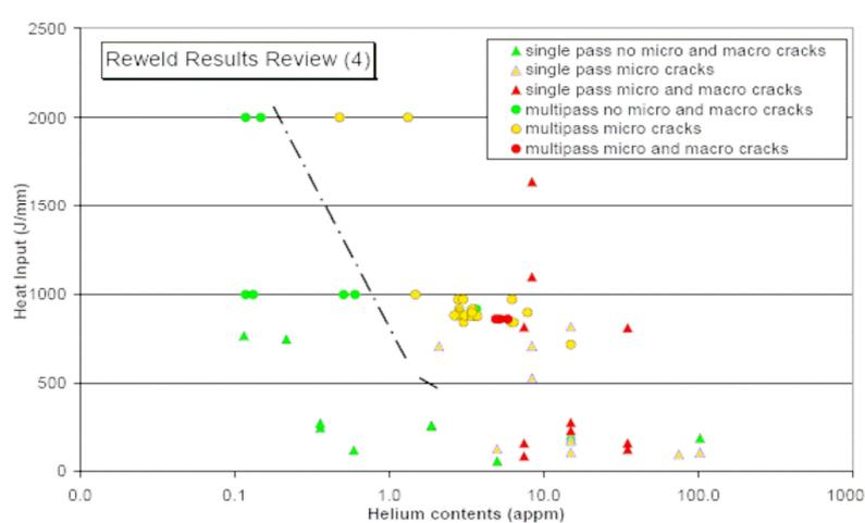
Figure 3 The appearance of cracks in welds of type 316 as dependent on welding heat input and helium content of the steel after irradiation in the HFR, Petten.
