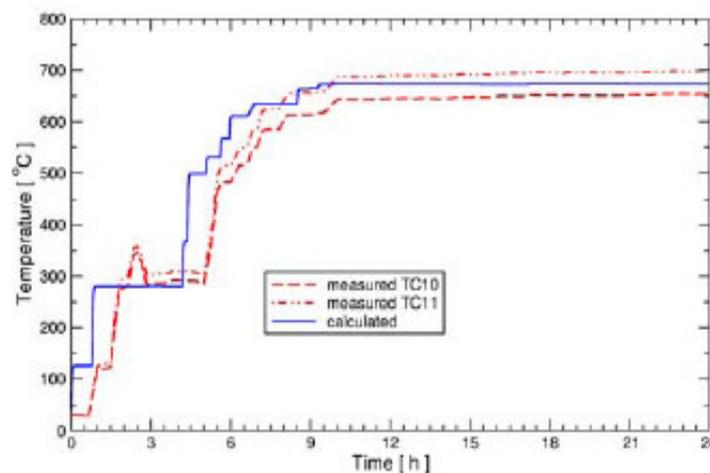
Figure 1 Predicted and measured temperatures in the ceramic breeder bed of the PBA as dependent on the time after neutron irradiation start-up.
