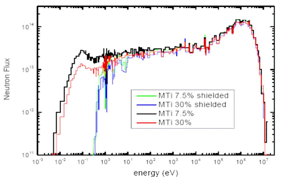
Figure 5 The effect of shielding on the neutron spectrum exposure of meta-titanate with different  ${}^6\text{Li}$  contents.
