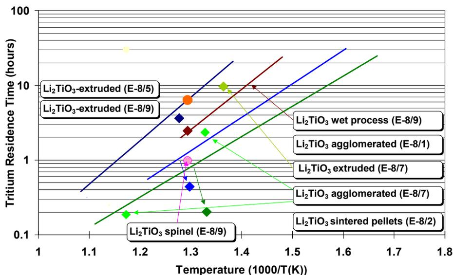
Figure 4 Tritium residence times for lithium meta-titanate  $\text{Li}_2\text{TiO}_3$  pebbles irradiated up to about 17 % total lithium burn-up in the HFR, Petten.
