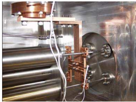
Figure 3. The pellet injector cavity built at O.R.N.L.
