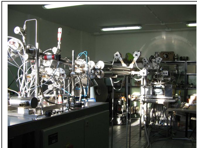
Figure 2. The Ignitor Pellet Injector propelling sub-system built by ENEA at Criotec Impianti.
