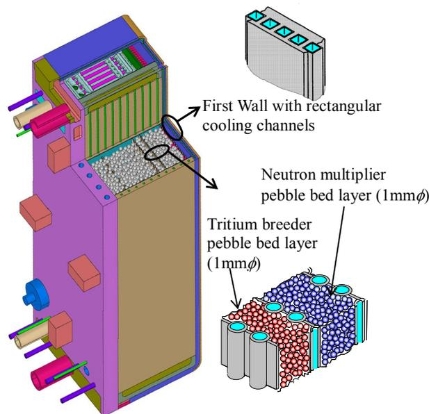
*FIG. 1. Structure of Water Cooled Solid Breeder TBM [3].*
