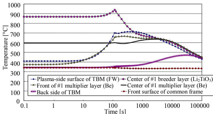
FIG. 3. Temperature transient of TBM, pipe break in TBM.
