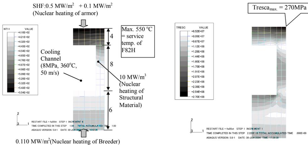
(1) Temperature distribution in the cross section of first wall of the HCSB TBM
