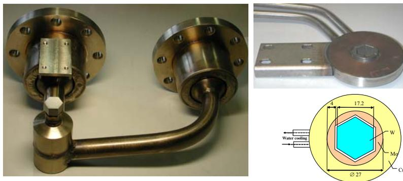
**Fig. 4:** Target device with mock-up holder and water-cooled shielded mask.
