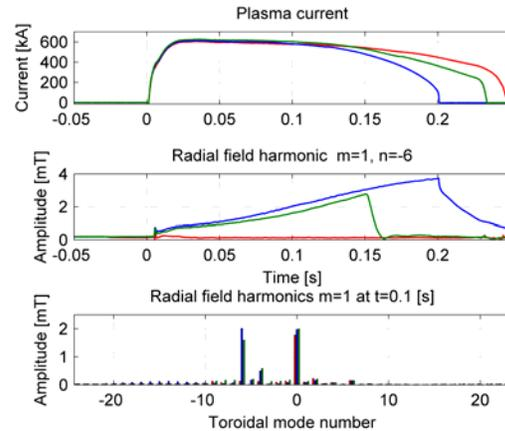
FIG. 9. Feedback control on RWMs. Comparison among pulses programmed with same parameters, but differing in RWM control.
