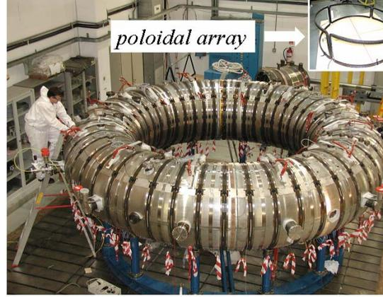
FIG. 2. Assembly of saddle coils on mechanical structure. Top right corner shows a poloidal array consisting of four saddle coils.
