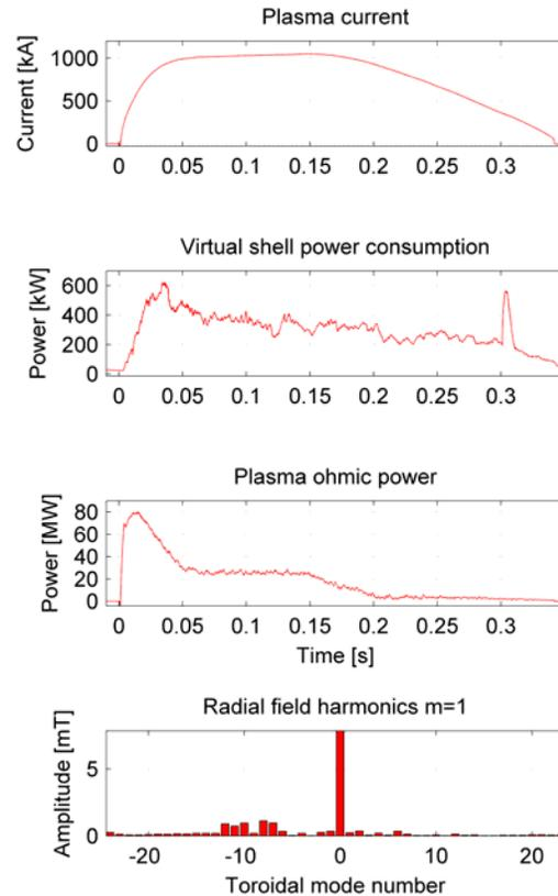
FIG. 10. Power consumption associated to MHD mode control
