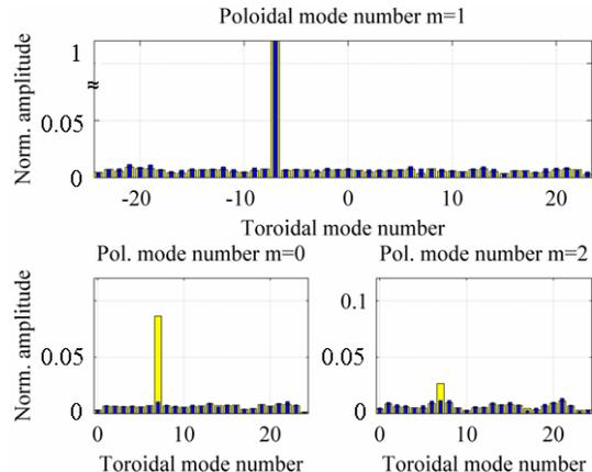
FIG. 7. Generation of  $m=1$   $n=7$  mode. Magnetic field spectra obtained without (yellow) and with decoupling (solid).
