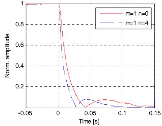
FIG. 8. Cancellation of disturbance  $m=1$   $n=0$  and  $m=0$   $n=4$  modes produced by field shaping and toroidal windings, respectively
