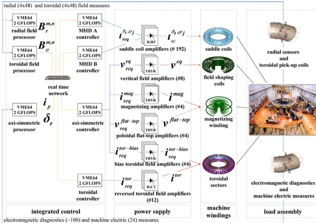
FIG. 4. Layout of the RFX-mod plasma control system.
