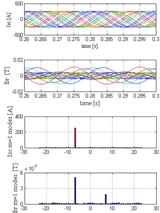
FIG. 3. Open loop generation of  $m=1$   $n=-7$  mode. From above to below: currents and radial field in the poloidal arrays located at the toroidal coordinate  $0 \leq \varphi \leq \pi/8$  rad;  $m=1$  spectra for current and radial field.
