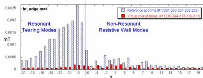
FIG. 1.  $m=1$  toroidal Spectra of  $Br$  at sensors with (red) and without (blue striped) mode control.
