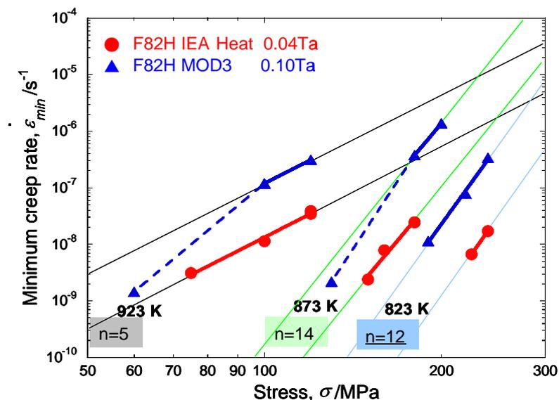
FIG.4 Stress dependence of minimum creep rate of F82H-IEA heat and F82H Mod3 (F82H with 0.1Ta, low Ti, N).  $\epsilon_{min} = A\sigma^n$ , where A is constant, s is stress, and n is stress exponent.
