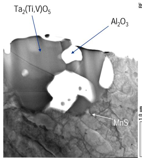
FIG.6. Cross sectional bright field STEM image of complex inclusion found in F82H
