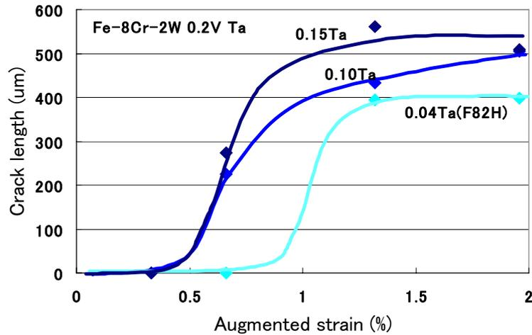
FIG.5. Ta concentration dependence of hot cracking susceptibility obtained by trans- varestraint tests
