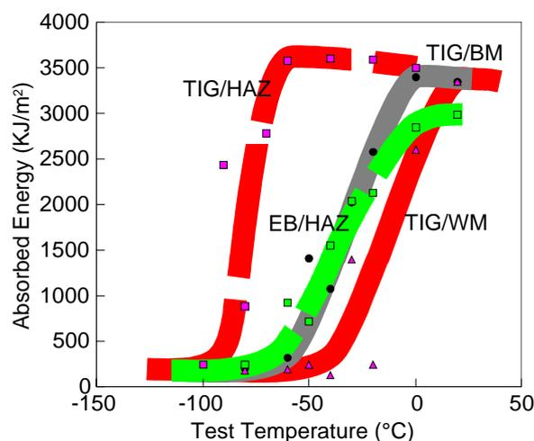
FIG.1 The Charpy impact tests on TIG/EB weldments of F82H. BM: Base metal, WM: Weld metal, and HAZ: Heat affected zone.
