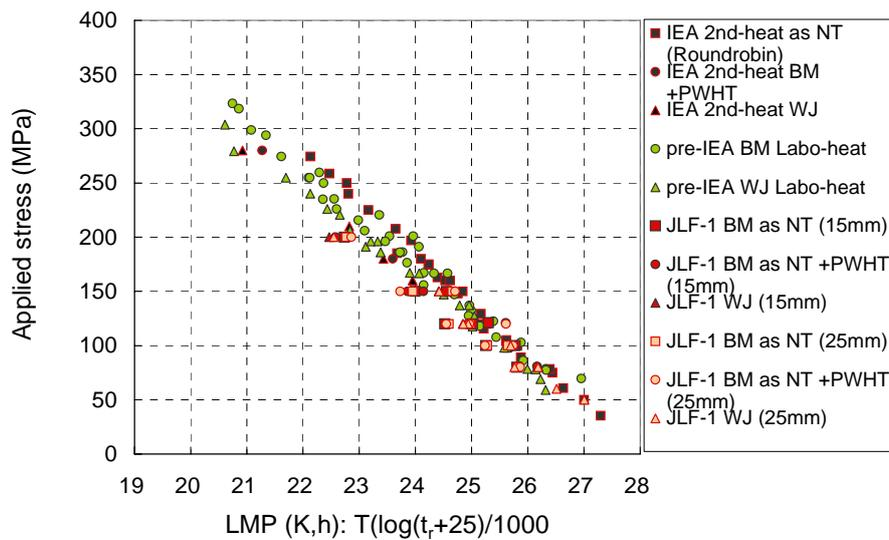
FIG.2. The creep tests on base metal and TIG weldments of F82H and JLF-1
