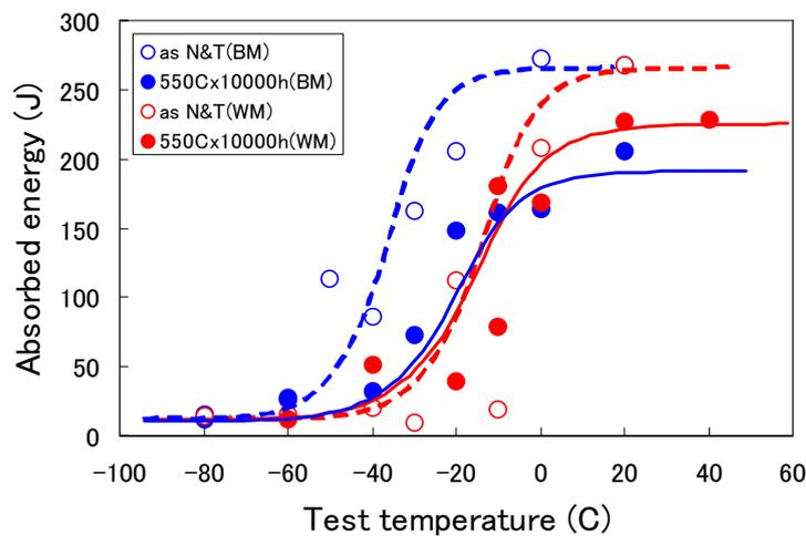
FIG.3. The Charpy tests on aged base metal and TIG weldments of F82H
