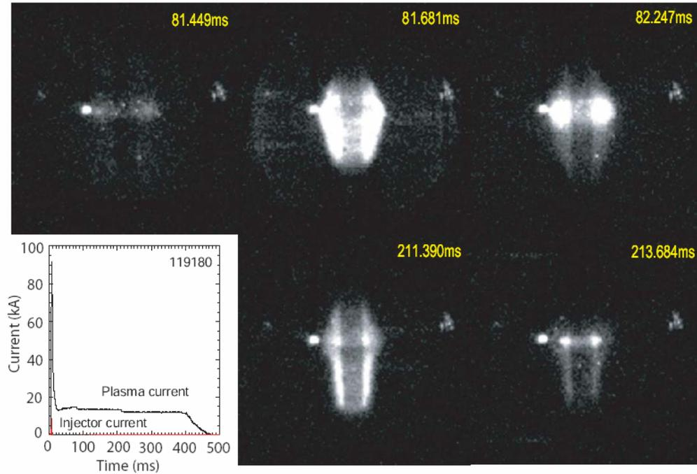
*Figure 4: Fast camera images and plasma and injector current for a discharge that persisted for 400 ms. At 400 ms, the current in the poloidal field coils was ramped down to zero. At about 81 ms and 211 ms, the plasma discharge contacts the center stack resulting in visible emissions. Note that the plasma current drops after each contact with the wall. During the rest of the phase, the visible emission is very low, similar to that in the image at 81.449 ms*
