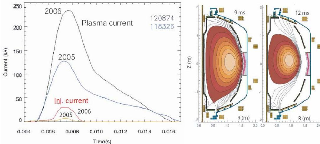
Figure 3: Plasma current injector current from discharges during 2005 and 2006. Operation at higher capacitor bank voltages and at higher values of the injector and toroidal flux resulted in the increase in the closed flux current to 160 kA during 2006. Equilibrium reconstructions at 9 and 12 ms for the higher current discharge (shot 120874) show the production of a closed flux equilibrium.
