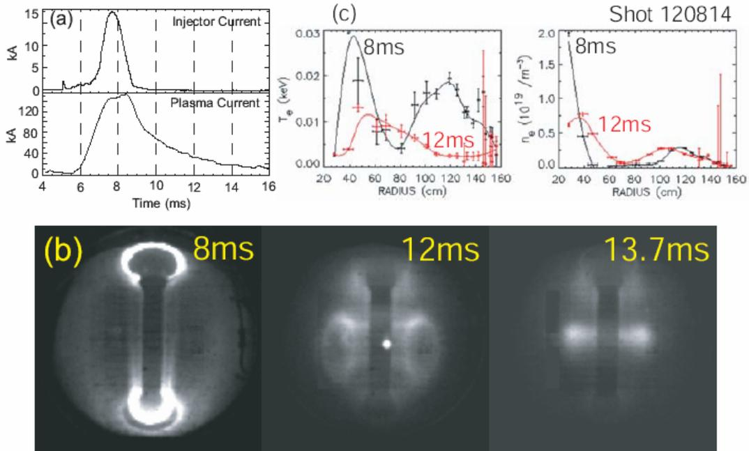
Figure 2: Shown are (a) the plasma and injector current traces (b) fast camera images and (c) the electron temperature and electron density profiles, at 8 and 12 ms from a CHI discharge in NSTX. The small bright glow near the middle of the vessel is light from a tungsten filament located near the wall inside the vessel.
