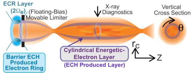
FIG. 4. Experimental configuration for radial transport barrier formation by the use of off-axis barrier ECH.
