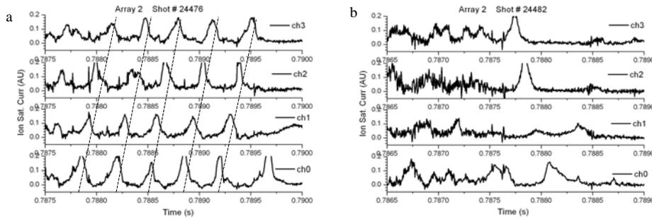
*Fig 3 Signals from array 2 probes. (a) Signals with the divertor on but the x-point 0.015 m outside the vacuum vessel. (b) Signals with the divertor on and the x-point 0.012 m inside the vacuum vessel*
