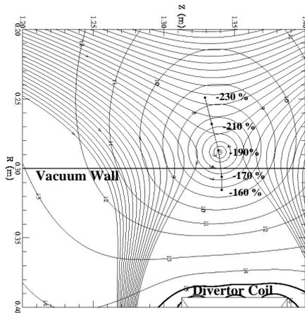
Fig. 2. Close up view of the divertor region for the west end divertor as in Fig 1. For a divertor current of  $-190\%$ , the x-point is  $\sim 0.012$  m inside the wall. The other points show the x-point location for several other currents.
