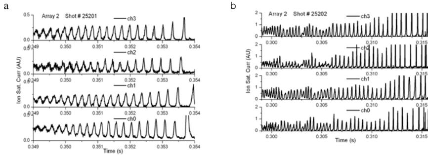
Fig 4. (a) Shot 25201 without Kinetic Stabilizer plasma. (b) Shot 25202 with Kinetic Stabilizer plasma. The  $m = -1$  signal duration is longer for shot 25202 with the KS on.
