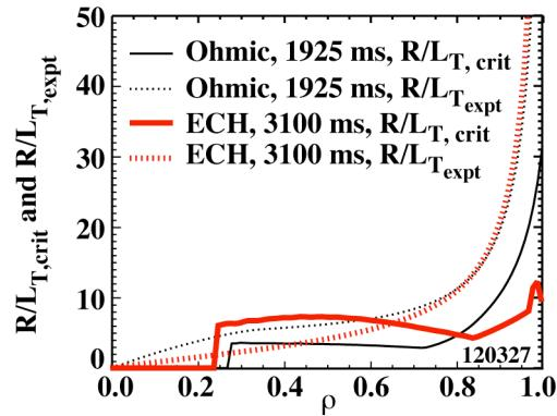
FIG. 6. Comparing SOL of theoretical prediction of ETG critical gradient and experimental gradient. The critical gradient is exceeded for most of the outer half radius in both heating conditions.
