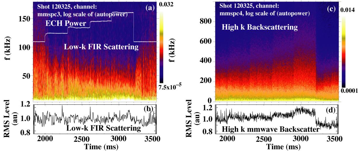
FIG. 3. Low  $k$  frequency spectra narrow (a) and fluctuation levels (b) are constant or decrease during ECH. In contrast, high  $k$  spectra broaden (c) and fluctuation levels (d) increase.
