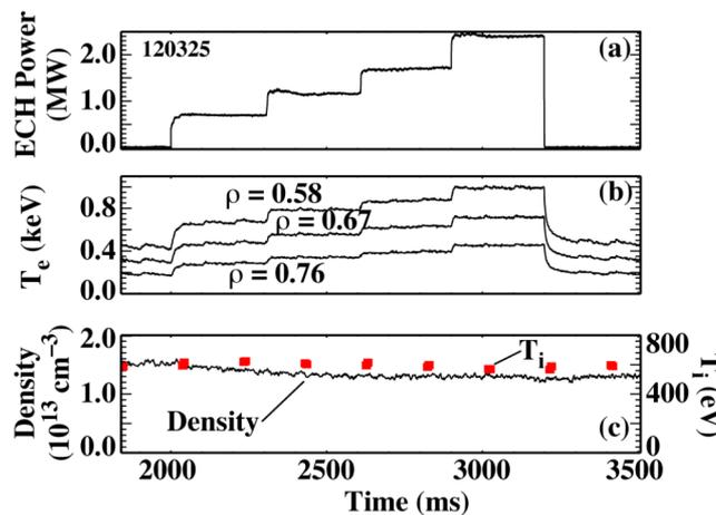
FIG. 1. (a) ECH heating, (b) electron temperature at different radii showing increase with ECH, (c) density and ion temperature ( $r/a \sim 0.4$ ).
