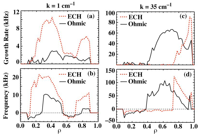
FIG. 5. GKS predictions of growth rates and real frequencies for two different wavenumbers (a,b)  $1\text{ cm}^{-1}$  and (c,d)  $35\text{ cm}^{-1}$  for two times: Ohmic (solid line) and ECH (dotted line) heating.
