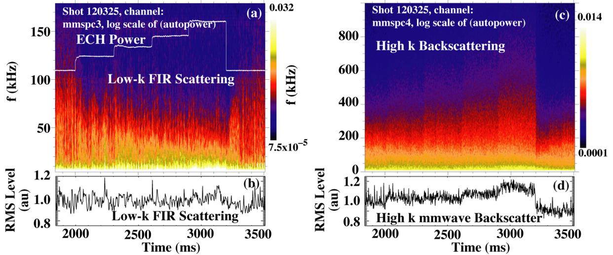
FIG. 3. Low  $k$  frequency spectra narrow (a) and fluctuation levels (b) are constant or decrease during ECH. In contrast, high  $k$  spectra broaden (c) and fluctuation levels (d) increase.
