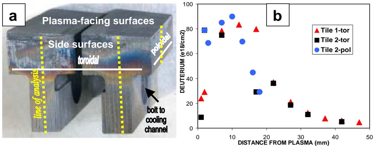
Fig. 3. Mk-I CFC tiles with flaking co-deposits (a) and the distribution of deuterium on surfaces in gaps between the tiles (b).
