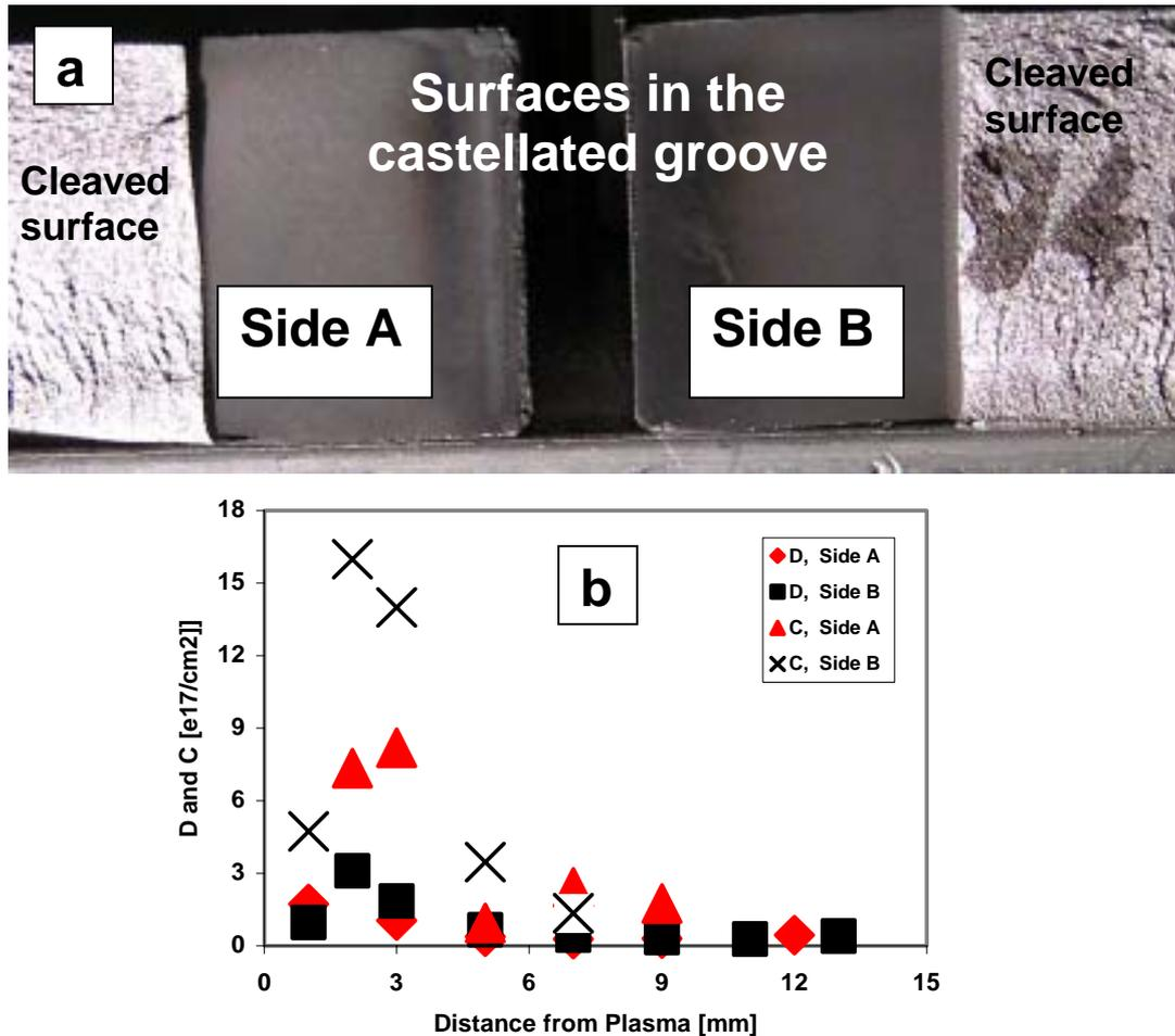
Fig. 2. Deposition pattern (a) and deposition profiles of deuterium and carbon (b) inside the castellated groove of the beryllium belt limiter tile.
