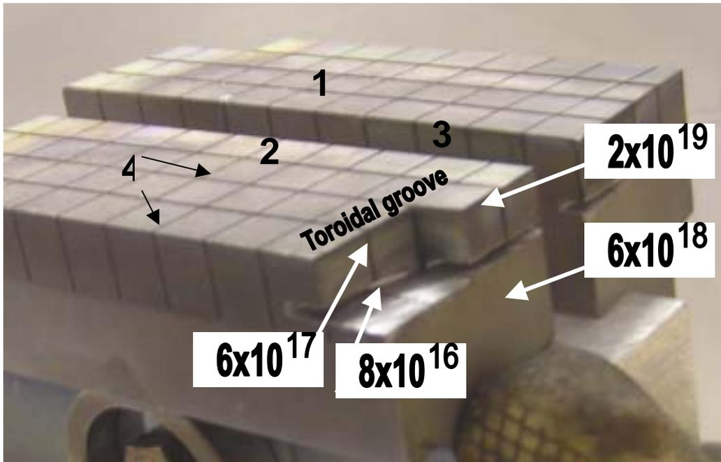
Fig. 4. Roof-shaped beryllium tiles of the Mk-I divertor: upper (1) and lower edge with an area shadowed by the adjacent higher tile (2); poloidal gap between tiles (3); castellated grooves (4). Deuterium content on the side surfaces and in castellated grooves on the Mk-I beryllium tile is indicated.
