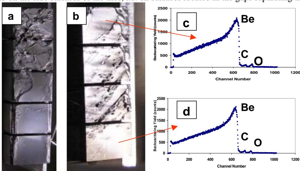
Fig.1. Plasma-facing surfaces of castellated beryllium tiles of the belt limiter (a) and (b); EPS spectra showing surface composition in two locations on the tiles (c) and (d).
