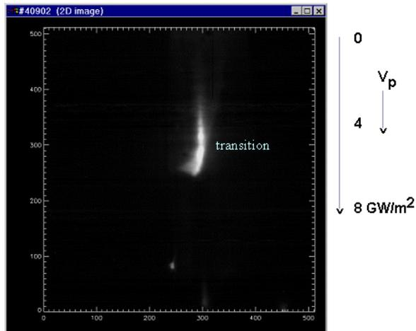
Fig.3. Track of lithium pellet showing the transition from atomic to cluster/droplet erosion.
