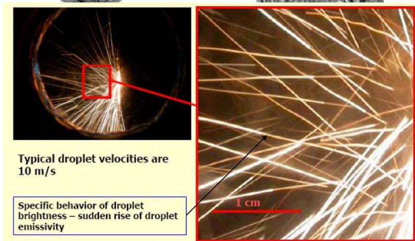
**Fig. 2. Photo of tungsten surface erosion in dust producing regime in QSPA.**
