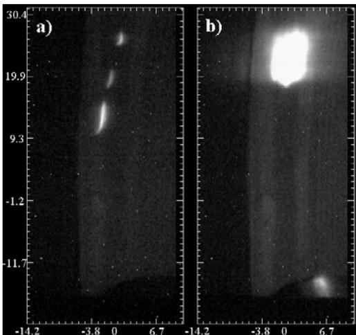
Fig. 5. Photo of carbon dust cloud forming virtual limiter in T-10.
