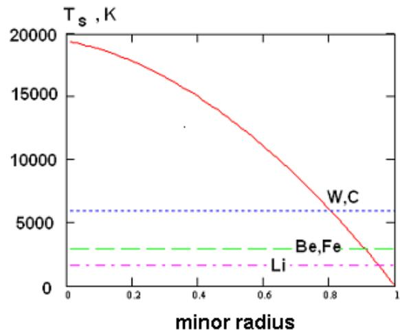
Fig 4. Profiles of the plasma parameters in T-10 and survival domains for Li, Be, Fe, W, C.
