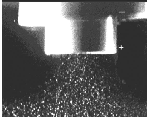
Fig.6. Photo of radioactive dust evacuation by means of electric fields.
