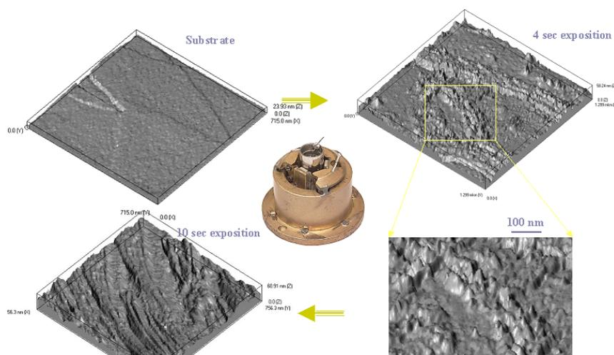
**Fig. 1. View of the in-situ STM and surface evolution after exposure in T-10.**
