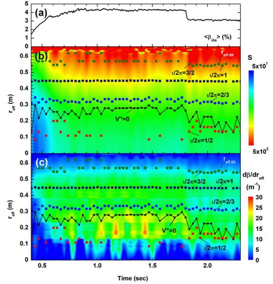
FIG.3 Temporal changes of (a)  $\langle\beta_{\text{dia}}\rangle$ , (b)  $S$ , and (c)  $d\beta/dr_{\text{eff}}$  in the entire plasma, and the comparison with radial positions of plasma boundary, several resonant surfaces and  $V''=0$ .
