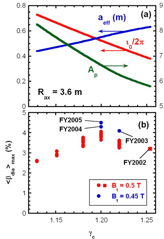
FIG.1 Changes of (a)  $a_{\text{eff}}$ ,  $t_0/2\pi$ ,  $A_p$  and (b) achieved  $\langle\beta_{\text{dia}}\rangle$  as a function of  $\gamma_c$ .
