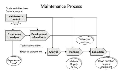
FIG. E.1. Maintenance process.
