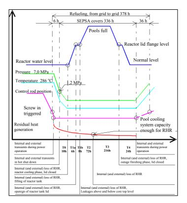
FIG. A.4. Thermal hydraulic analyses, made during the SEPSA project, showed that all operating modes with critical reactor should be included in power operation mode PSA.
