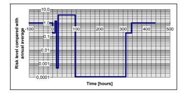
FIG. A.5. Risk level during the refueling outage as a function of time.
