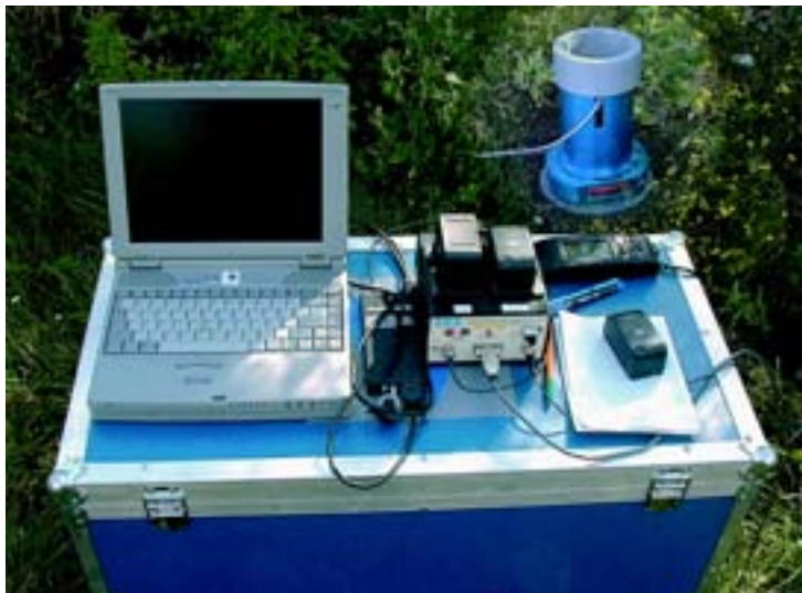
FIG. 3. In situ element determination in soil by XRF spectrometry.
