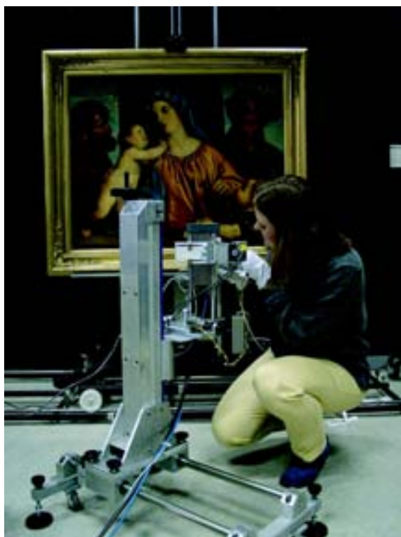
FIG. 4. Pigment analysis with portable XRF spectrometer.
