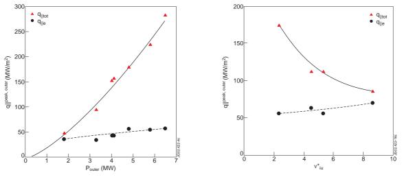
Figure 3(a) Peak parallel power measured at the outer target vs. heating power at constant density and (b) peak parallel power vs. upstream SOL collisionality at constant input power (12MW)
