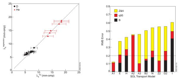
Figure 4(a) Outer power decay length in helium and deuterium discharges plotted against the scaling of equation (2). (b) RMS difference in scaling exponent against top ten models - classical A1, neo-classical A3, MHD interchange E, drift ballooning turbulence H, classical electron conduction A3, Bohm N, poloidal gyroradius N, endplate MHD B2&G2 and skin depth I. Experimental error is estimated to be  $\sim 0.2$ .
