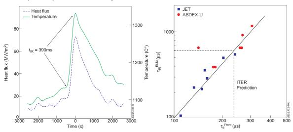
Figure 5(a) Time evolution of peak power and temperature at the JET divertor during a type I ELM [15]. (b) Scaling of ELM rise time  $\tau_{IR}$  with ion parallel transit time  $\tau_{I|} = 2\pi Rq_{95}/c_{sped}$  in JET and ASDEX-Upgrade [13]
