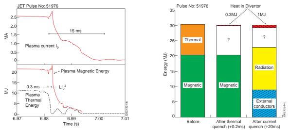
Figure 8. A JET disruption in which the thermal energy is lost in 0.3ms and magnetic energy over 20ms, (b) energy balance after thermal quench ( $\Delta W_{th} = 10MJ$ ) and after the loss of magnetic energy ( $\Delta W_{mag} = 20MJ$ ) disruption - question marks show unaccounted or unresolved contributions.
