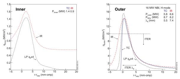
Figure 2. The extracted power profiles measured at the inner and outer divertor targets in an unfuelled type I ELMy H-mode(16MW) by a technique involving a slow sweep of the plasma over an embedded thermocouple (TC), infra-red camera (IR) and target Langmuir probes (LP). A power decay length  $\lambda_q$  of 5mm is assumed in ITER and the steady state surface power density is to be kept below 10MWm<sup>2</sup>.
