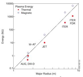
Figure 1 Stored energy increases with tokamak major radius as  $R^5$  and thus the average energy density during disruptions scales as  $R^3$ .
