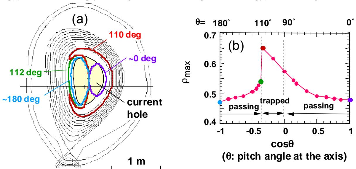
Fig.4. (a) Deuterium ion orbits with temperature 8keV and different pitch angle at the magnetic axis. (b) Maximum radial excursion of ions with different pitch angle started from the magnetic axis.
