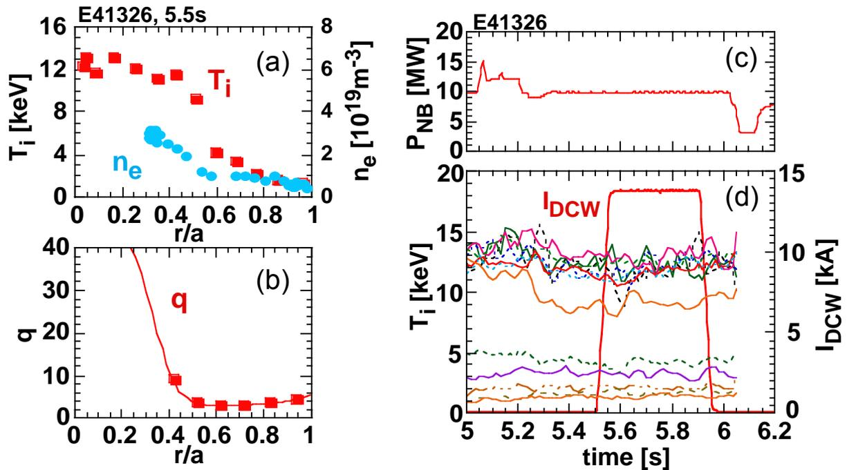
Fig.5. Application of an error field (DCW) to the Current Hole  $I_p = 1.4 \text{ MA}$ ,  $B_t = 3.7 \text{ T}$ ,  $q_{95} = 4.4$ ,  $\beta_N \sim 0.8$ . (a) Ion temperature and electron density profile. (b) Safety factor profile. (c) Time evolution of NB power. (d) Time evolution of ion temperature at several points and DCW coil current.
