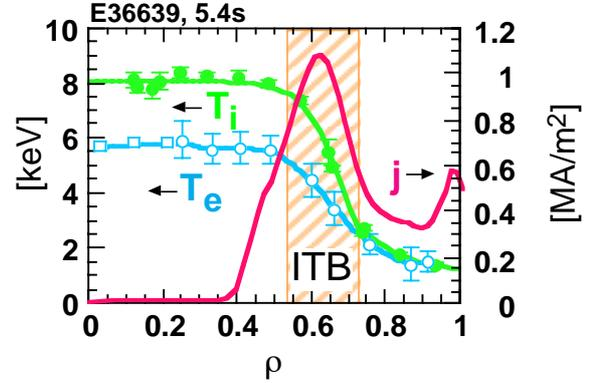
Fig.3. Temperature profiles and current density profile at 5.4 s of the discharge shown in Fig.2.
