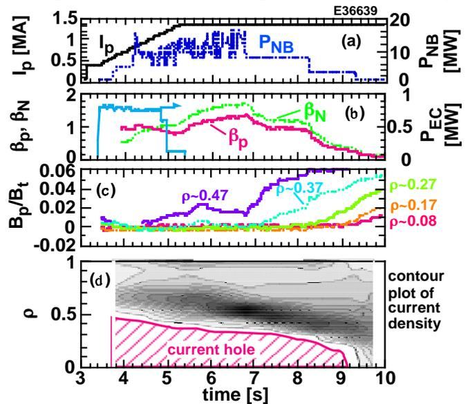
Fig. 2. Waveforms of a discharge in which the Current Hole was sustained for several seconds. (a) Plasma current ( $I_p$ ) and NB power ( $P_{NB}$ ; dotted line). (b)  $\beta_p$  (solid line),  $\beta_N$  (dotted line) and EC power ( $P_{EC}$ ; solid line). (c)  $B_p/B_t$  at the MSE measurement points. (d): contour plot of current density, where darker regions have a larger current density. The region of the Current Hole is indicated by a hatched area.
