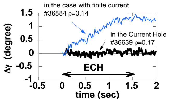
Fig.6. Waveforms of MSE measured pitch angle. Thick line shows the case with Current Hole and thin line shows the case with finite current of about  $0.3\text{MA/m}^2$  at the center. The time of zero is the start time of ECH.
