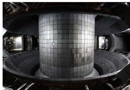
FIG. 5. PFC system with graphite tiles after completion in the vacuum vessel
