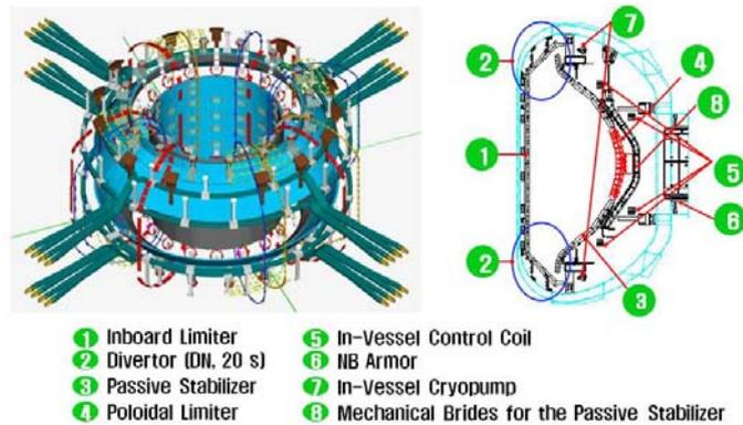
FIG. 1. KSTAR In-vessel components
