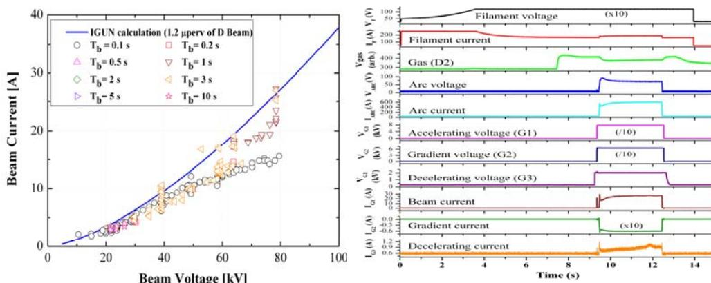
FIG. 11. (Left) The beam perveance data and (right) the waveforms of the 3-s beam extraction with the beam energy of 80 keV and the beam current of 27 A.
