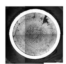
Carbide Pu fuel irradiated in Phenix FR
