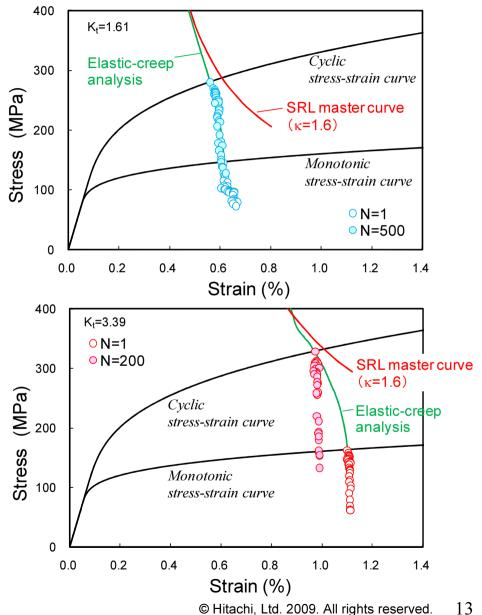
The stress redistribution locus (SRL) method was investigated experimentally in order to improve and rationalize creep-fatigue damage evaluation methods in the high temperature design rule of fast reactors.
