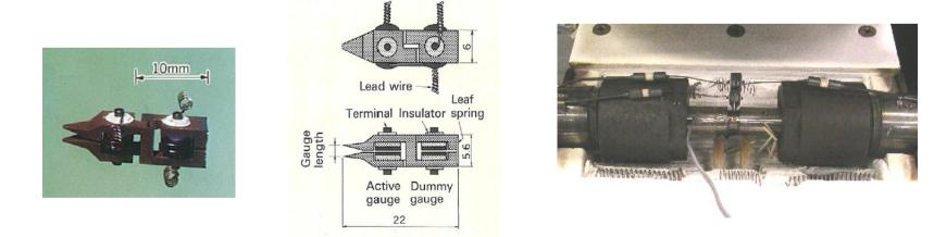
Capacitance type high temperature gage: Strain Pecker
