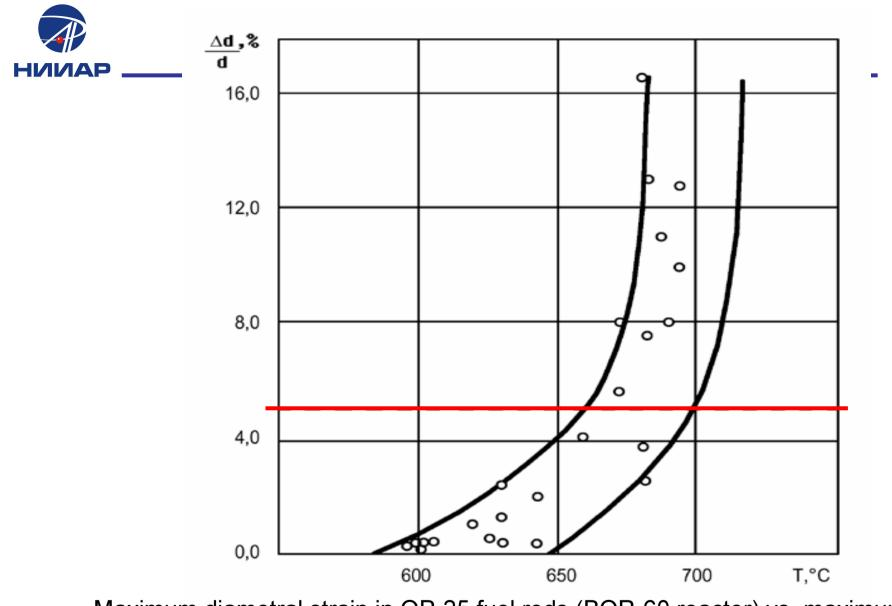
Maximum diametral strain in OP-25 fuel rods (BOR-60 reactor) vs. maximum initial irradiation temperature (--- level of maximum allowable form change)
