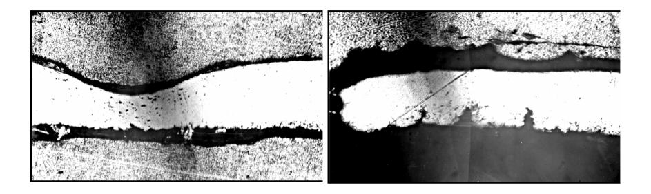
Typical areas of local thinning damage areas and several non-through ruptures of the cladding in the upper part of the fuel rods
