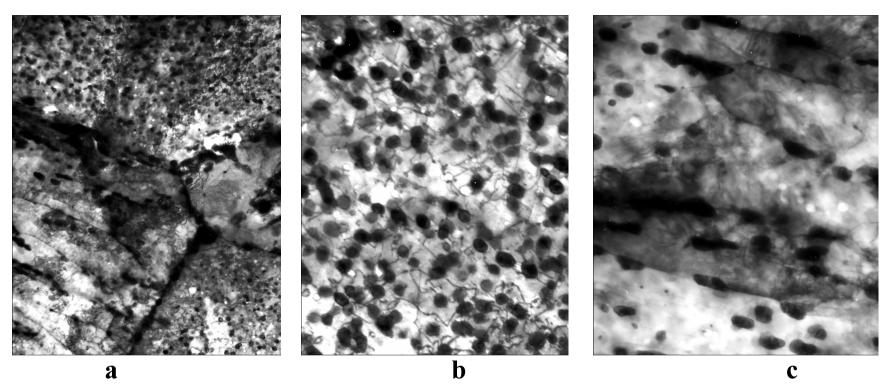
Structure of EP-450 steel as cladding material for BS-007 fuel rods irradiated in BOR-60 reactor (a – general view, x20000; b –voids, dislocation network and χ -phase precipitates in ferrite, x40000; c – voids and secondary phase precipitates in sorbite, x40000
