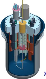
Expertise has been gained in the EU on Heavy Liquid Metal technology (Lead-Bismuth Eutectic – Lead) in the frame of R&D activities on transmutation of Long Lived radioactive waste using Accelerator Driven Systems (ADS)
