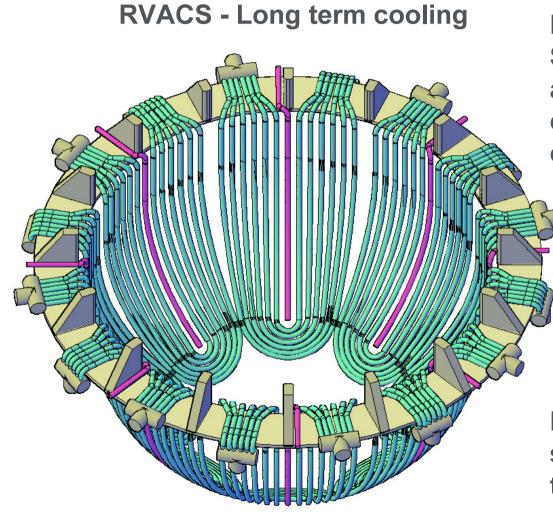
Reactor Vessel Air Cooling System connected to an inlet air collector and an outlet chimney to promote natural circulation.
