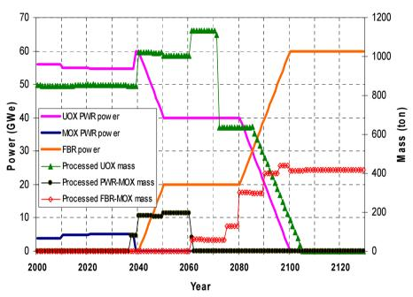
In this scenario, the total electric power remains constant (60 GWe) over the 21st century: PWRs decommissioned between 2040 and 2080 are replaced with FBRs
