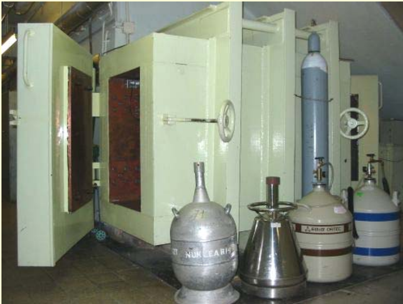
Low background iron chamber
