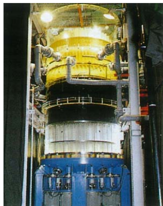
Hydraulic Test In Pressure Vessel
