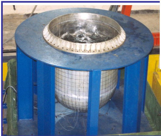
Shake table tests on RA model
