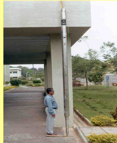
Fuel Sub assembly
