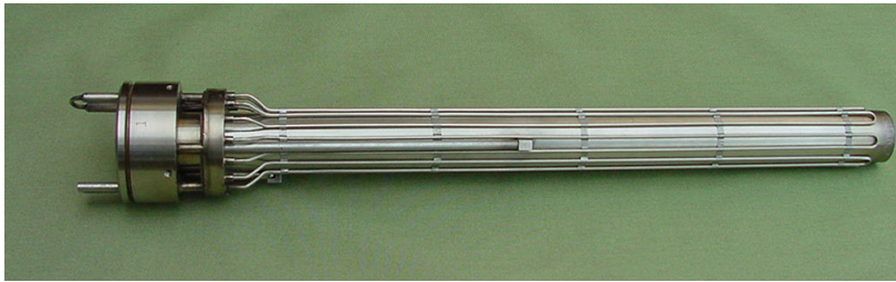
Cover gas hydrogen meter
