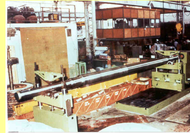
Primary pump - Shaft
