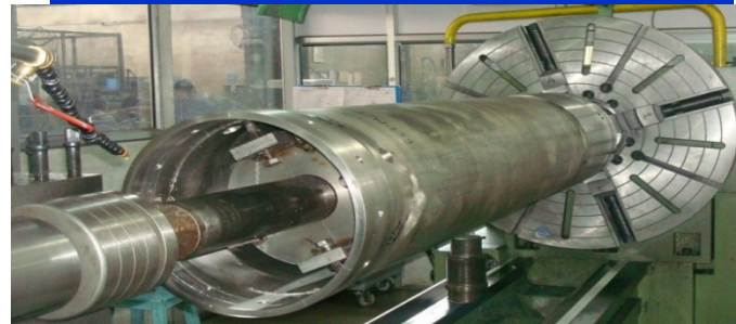
Primary sodium pump
