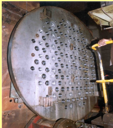
Grid plate sector Top plate rough machining
