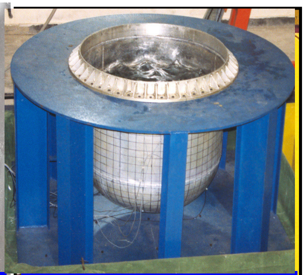
10 t Capacity Shake Table
