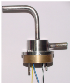
Semiconductor oxide based Compact hydrogen sensor
