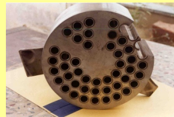
IHX Tube to Tube Sheet Joint Mock up
