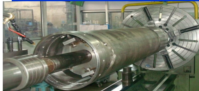
Primary sodium pump
