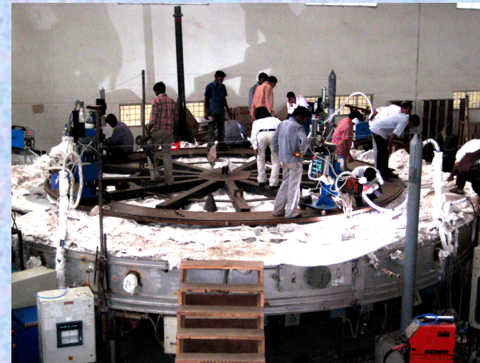
Hardfacing of PFBR Grid Plate
