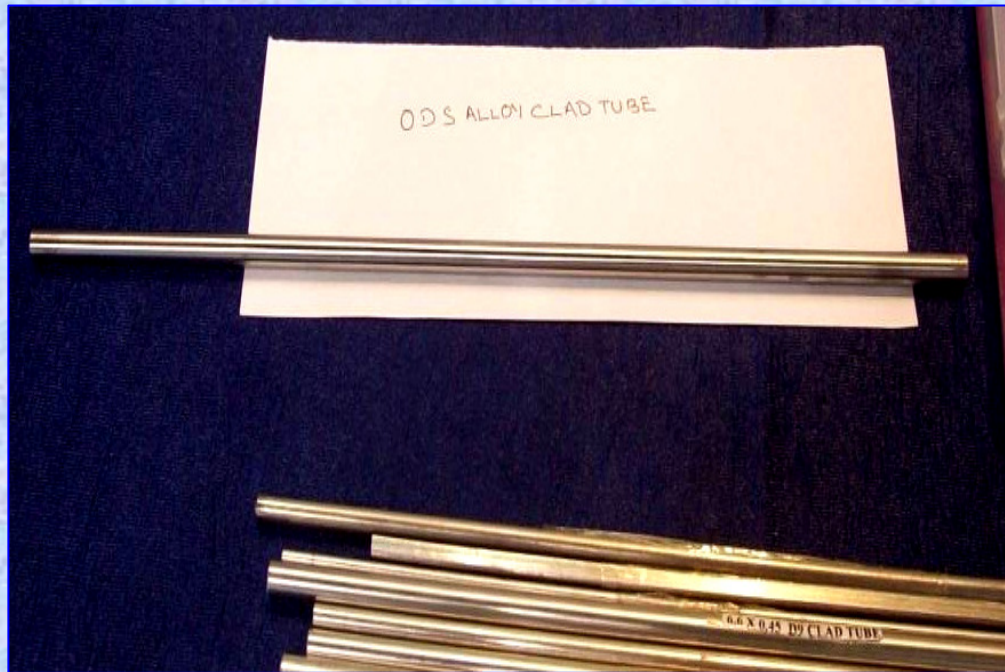
Clad tube (1.5 m) of 9Cr ODS ferritic-martensitic steel
