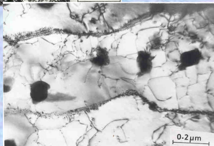
Subgrain development at 923 K
