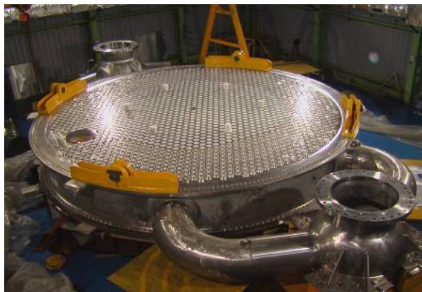
Grid plate with primary pipes
