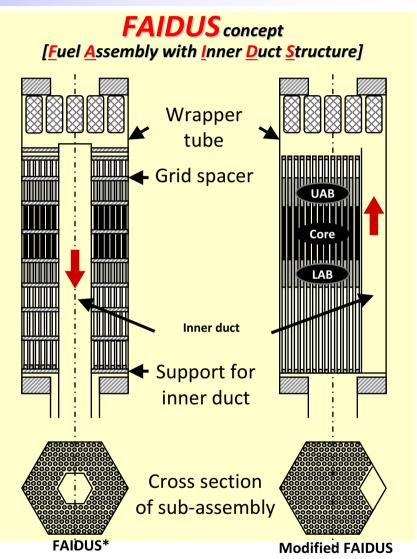
Fuel Assembly Designs Enhancing Fuel Discharge
