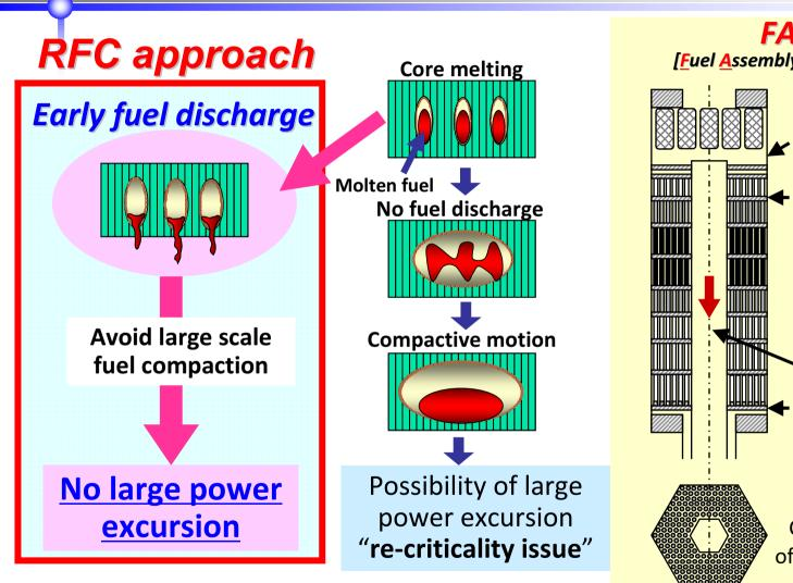
"Re-criticality free core" means that the fast reactor core which avoids severe energetics due to excursion in the course of core disruptive accident
