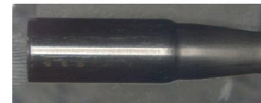
T91 end cap welded with magnetic pulse method
