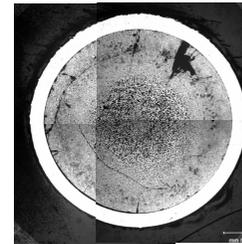
JRC/ITU Pu carbide fuel analysis
