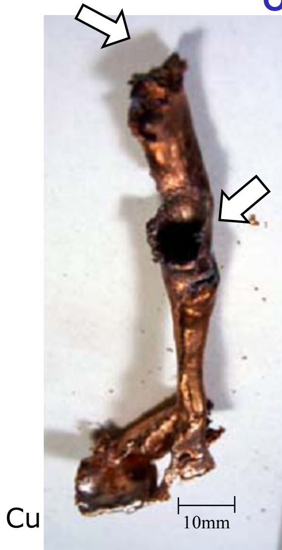
Fragment of Cu jet column with large-scale structure frozen in sodium pool ( T_{\text{sup}}: 16^{\circ}\text{C} , T_i: 1024^{\circ}\text{C} , We: 33 \sim 42 )
