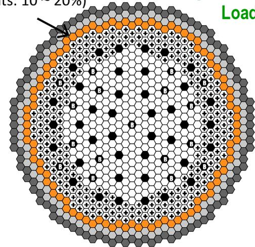
Reference Core Layout (12 Target Assemblies)
