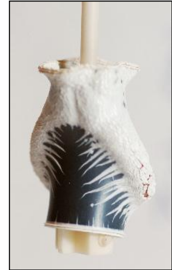
C: The clad behavior under air-steam oxidation
