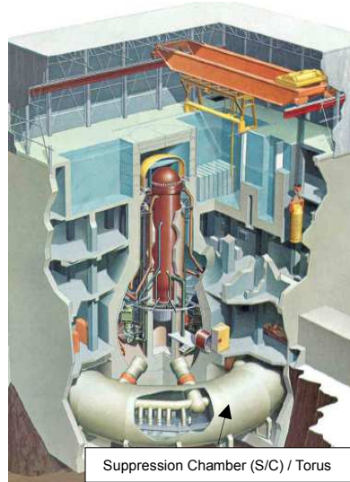
Suppression Chamber (S/C) / Torus Fukushima BWR with Mark I Containment
