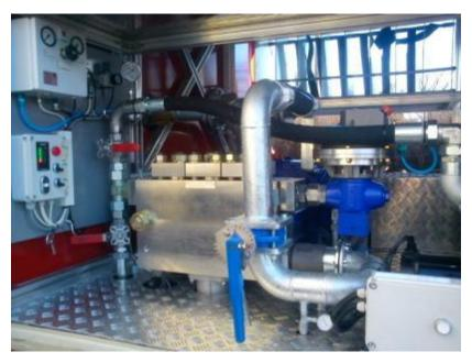
Volume flow Discharge pressure Power [m3/hr] 32 [bar] 70 [kW] 70
