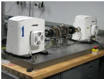
CIRFT test apparatus developed at ORNL CIRFT: Cyclic Integrated Reversible-bending Fatigue Tester
