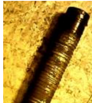
e6 top end cap & cladding surface [NNL]
