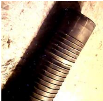
e1 top end cap & cladding surface [NNL]
