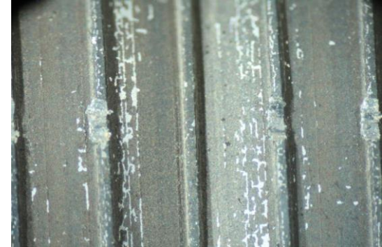
e6 top end cap & cladding surface [NNL]
