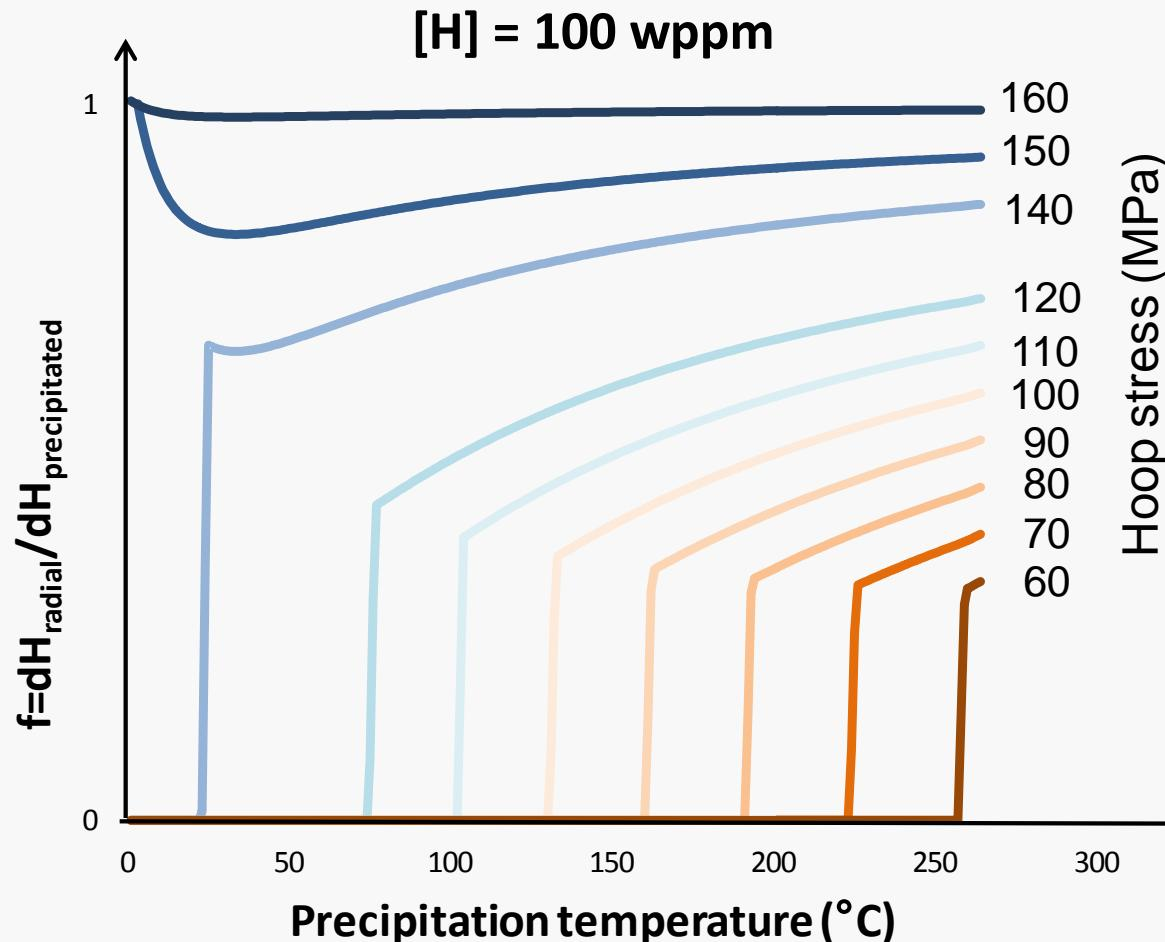
An assessment of the transient radial hydride precipitated fraction can be simply derived from post-test examinations
