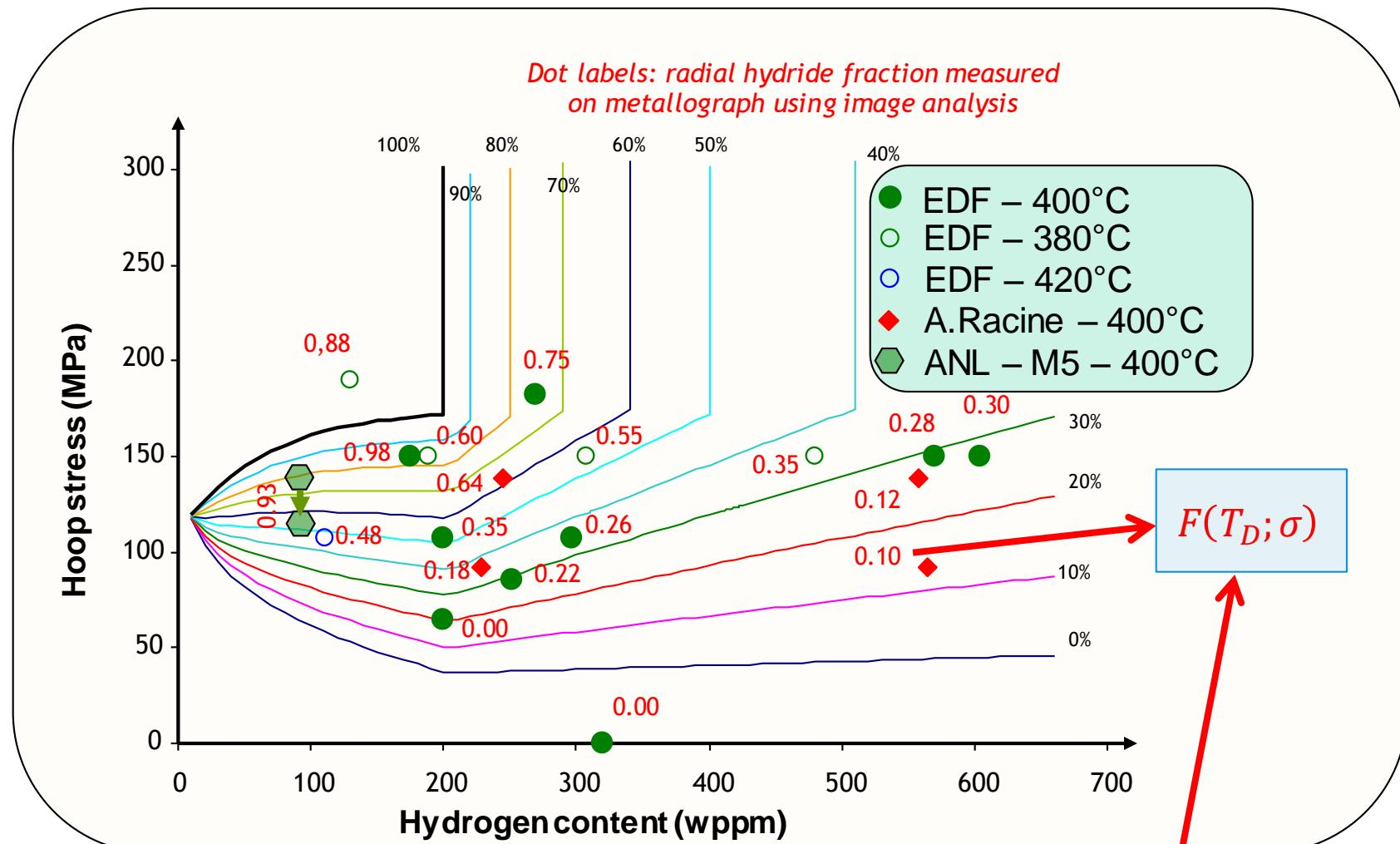
Linear interpolation provides a good assessment of post-test radial hydride fraction
