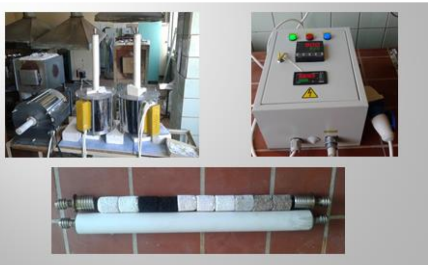
Experimental equipment for off gas treatment
